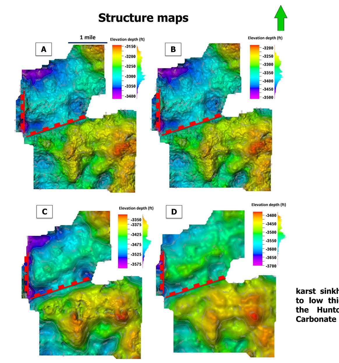
Figure 11. Surface structure maps in depth domain. A) Woodford structure map. B) Hunton structure map. C) Sylvan structure map. D) Viola structure map. Yellow lines indicate the locations of normal faults.
