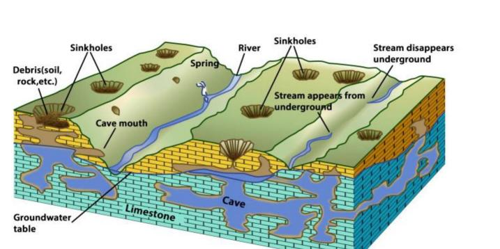
**Figure 4.** Generalized karst model including sinkholes, collapsed caves, and incised valleys. (Grotzinger and Jordan, 2010).
