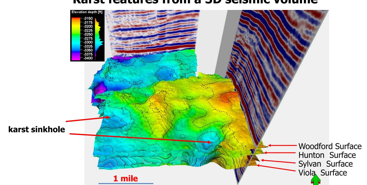
Figure 12. 3D view of the Woodford, Hunton, Sylvan, and Viola structure surfaces, showing low and high paleotopgraphies. The karst features, such as collapse and sinkholes on the Hunton unconformity surface are prominent factors controlling the paleotopography and deposition of the Woodford Shale. Sinkhole features range in diameter from 1150 to 2300 ft. and extend vertically to almost 300 ft.
