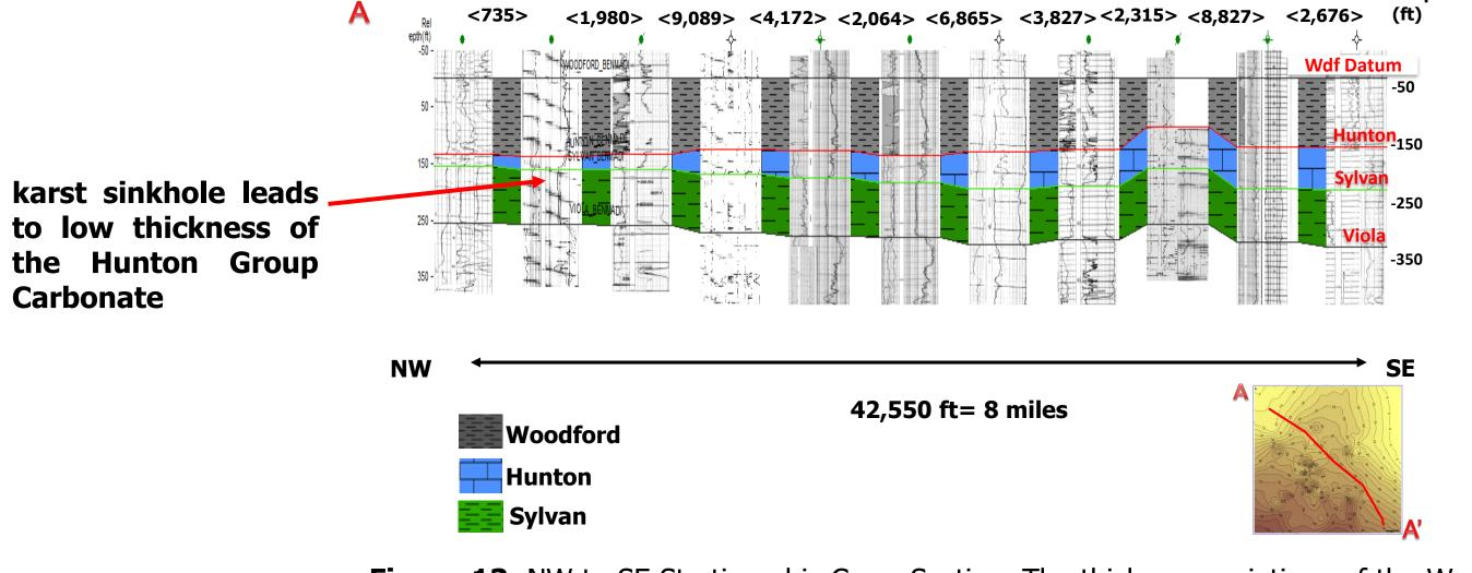
Figure 13. NW to SE Stratigraphic Cross Section. The thickness variations of the Woodford Shale are controlled by paleotopography of the underlying Hunton Group, where thicker Woodford is observed in the karst lows (sinkholes).
