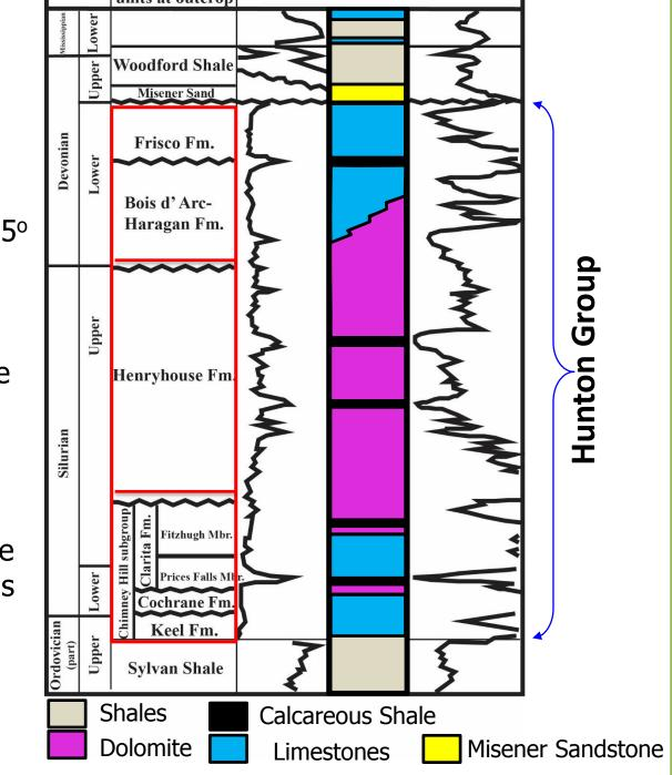
Figure 3. Hunton Group stratigraphic column in central Oklahoma with gamma ray (GR) and resistivity (R) type logs. This figure modified from Fritz and Medlock, 1994. The Misener Sandstone was added to this stratigraphic column as it was observed in the core and subsurface logs in the Cherokee Platform.
