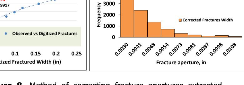
Figure 8. Method of correcting fracture apertures extracted from the Image J Software against the fracture aperture measured manually on the core site.
