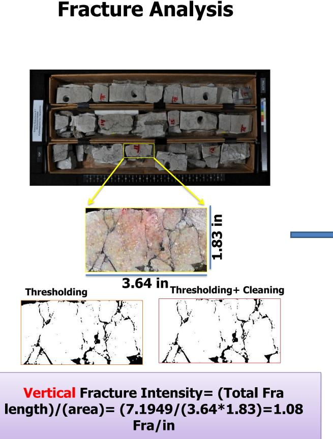
Figure 7. Fracture intensity analysis using Image J Software. First, we selected a specific area of the core, set the scale, enhanced the resolution of the picture by changing the saturations, and conducted thresholding. Next we cleaned the picture where we thought some features were not fractures when compared it with the original picture. Then we extracted the fracture length and width for the sample and calculated the fracture intensity per area as shown in this formula.
