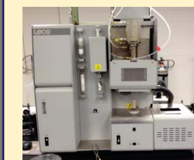
Figure 8. CS 230 Carbon Sulfur Analyzer.
