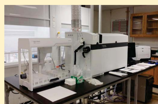
Figure 5. QQQ-ICP-MS (Model 8800) from Agilent Technologies (US). IDL can be as low as 0.02 pg/g, commonly around 1 pg/g. Therefore, it was used for low abundance trace elements determination.
