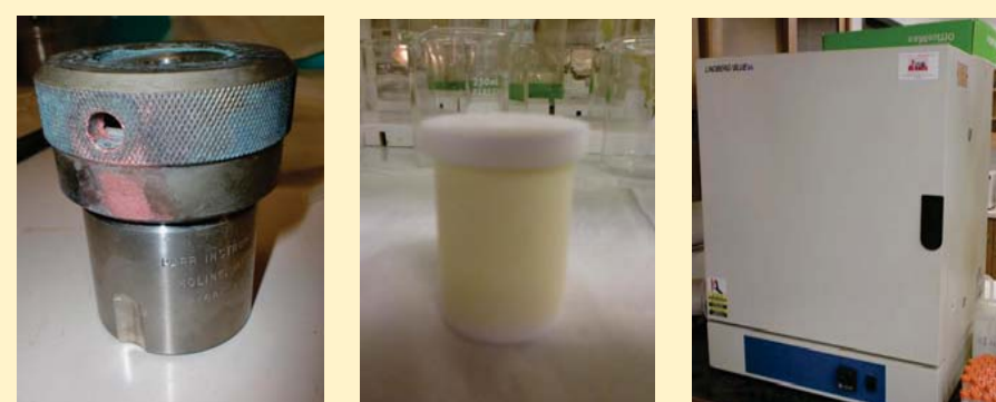
Figure 2. Operating temperatures and pressures up to a maximum of 250 °C and 1,800 psig are permitted in this vessel using a thick-walled PTFE liner. The maximum acceptable organic sample size is 100 mg to prevent venting based on our tests.
