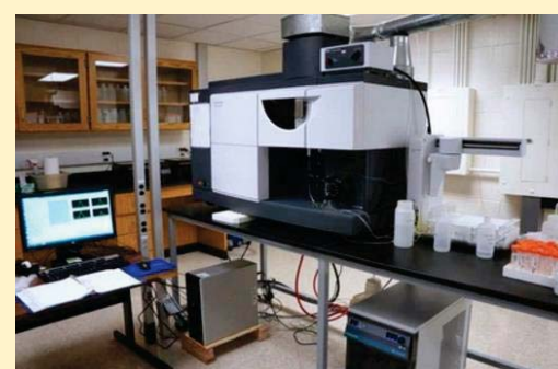
Figure 4. ICP-OES (Model 725) from Agilent Technologies (US). Instrumental detection limit (IDL) is about 2 ng/g commonly. Therefore, it was used for high abundance trace elements determination.
