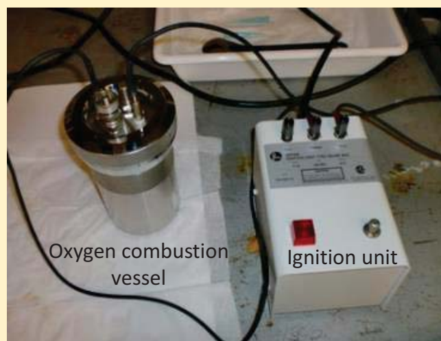
Figure 1. The oil sample inside the oil combustion vessel was ignited by an ignition unit (Model 2901 EB) that was connected to the vessel. The unit ignited the vessel by electrifying it. The combustion procedure is conducted inside a Covered Quartz Liner to prevent sample loss. vessel safely burns sample using oxygen charging pressures up to 40 atm. Generally, the maximum combustible material size is 1,100 mg of oil.
