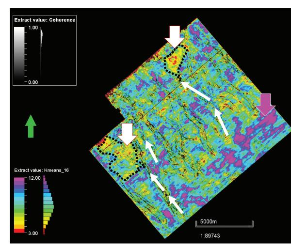
By using the combination of those attributes a K-means classification technique was used to identify facies. Following parameters where used for classification:
