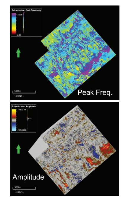
Horizon slices though the studied section. The scope of this study is the integration of several of the characteristics exhibit from seismic attributes by using statistical aproaches in a quick seismic classification.
