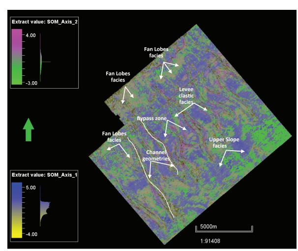
SOM classification technique was used. The latent space was selected in a color scale of 256 colors for allowing visualization. Parameters:
