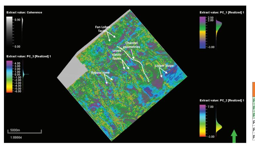
Combination of PC1, PC2 and PC3, allows a better interpretation of facies. The result is similar to the resulting image given for K-means technique. However, PC analysis interpretation. First 3 PC's reflect the 80% of the variability of the data. That is why the remaining PC components were not used.
