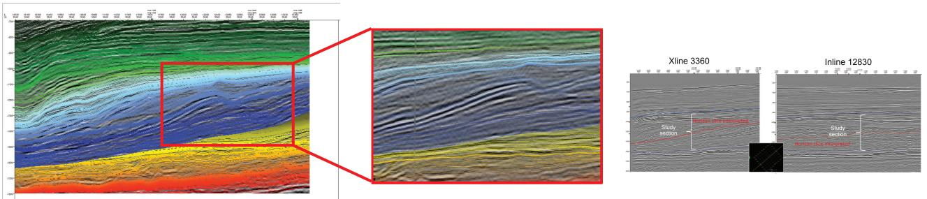
Horizon cube built to constrain the generated inversion model. Chronostratigraphic surfaces were generated using dip steering volume as source of the calculation. The resulting horizon surfaces follow pretty close the reflectors on the seismic information. These stratigraphic surfaces were used to build the low frequency model for the seismic inversion
