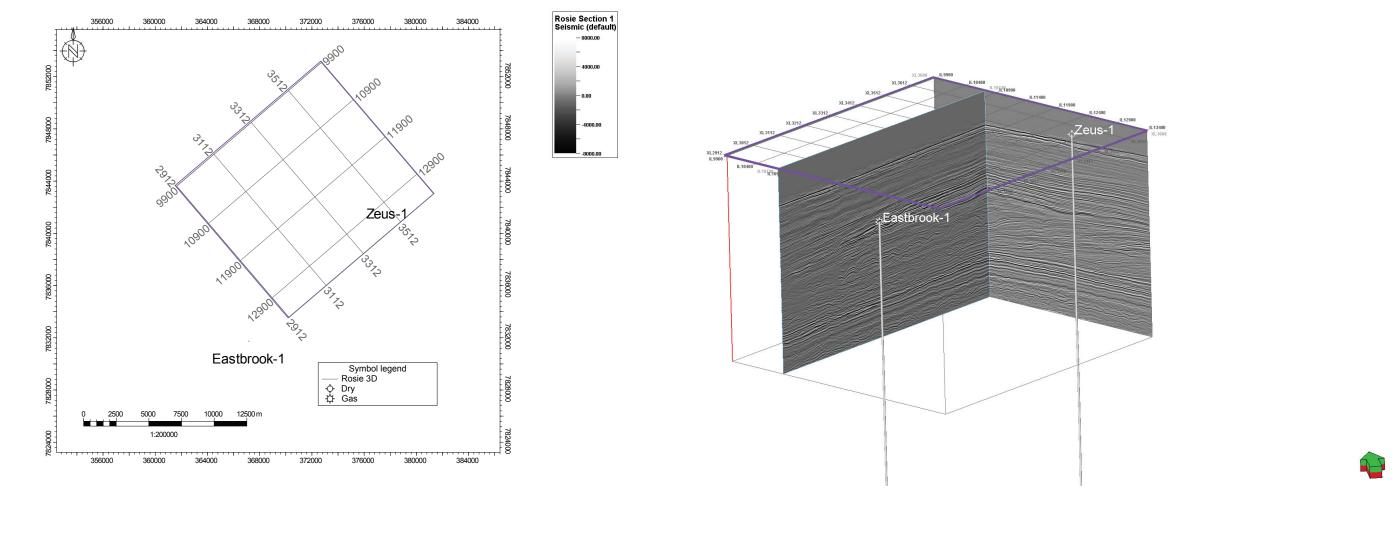
The study is based on seismic stratigraphic interpretation performed over the a section of the Rosie 3D volume, the integration with well log data, and attribute analysis.
