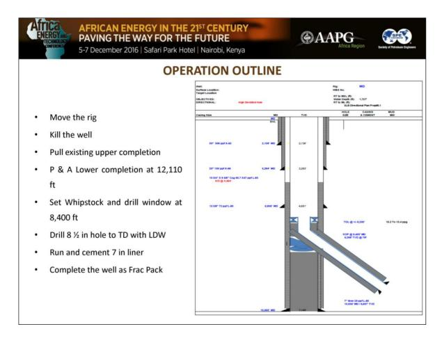
Presenter's notes: Upon completion of objectives, customer agreed the operational sequence having as critical points for the liner the whipstock setting depth and angle and the 8.5 in hole drilling. An operations overview of the complete intervention is as follows:
