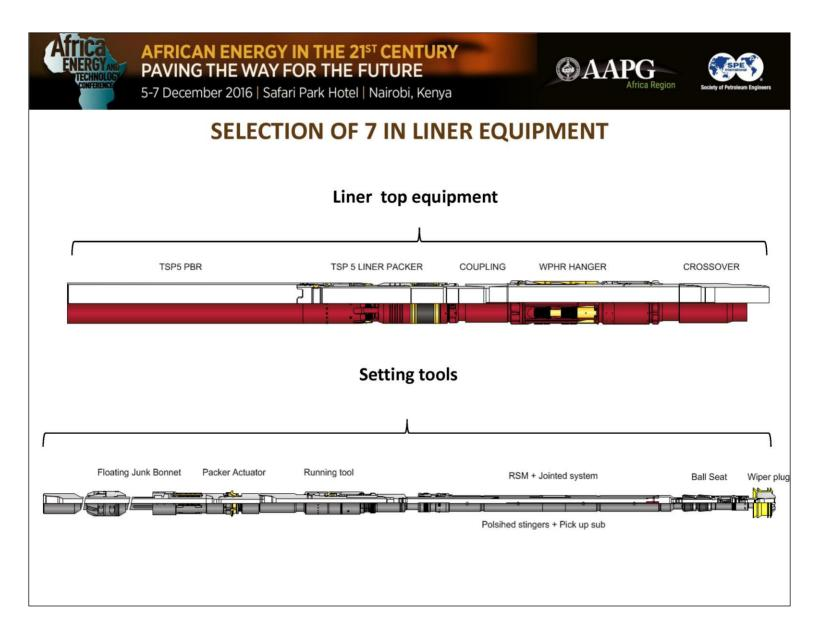
Presenter's notes: Here is a simple drawing of liner setting tools and liner equipment.
