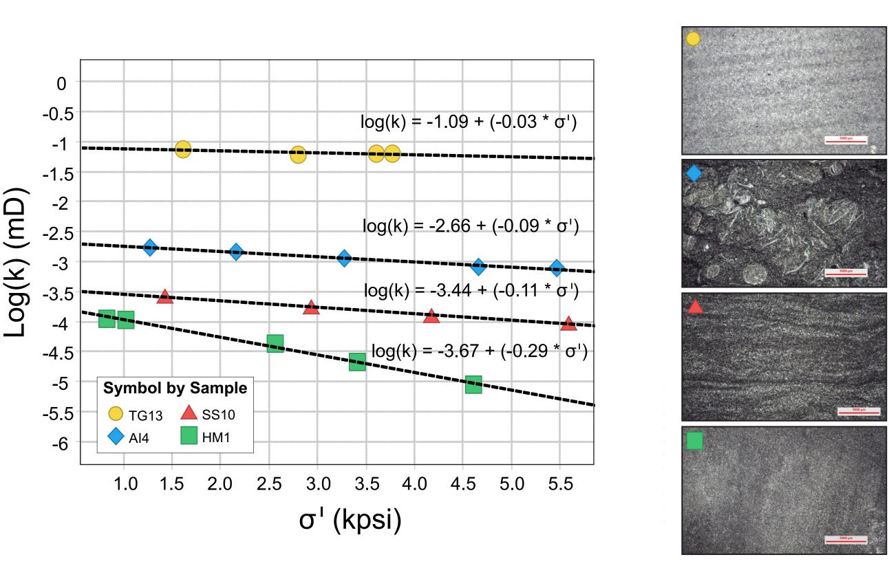
**Figure 11** - Log of permeability (k) versus effective stress ( $\sigma^{1}$ ), showing the wide range of permeabilities, as well as the difference in permeability sensitivity to stress across reservoir facies
