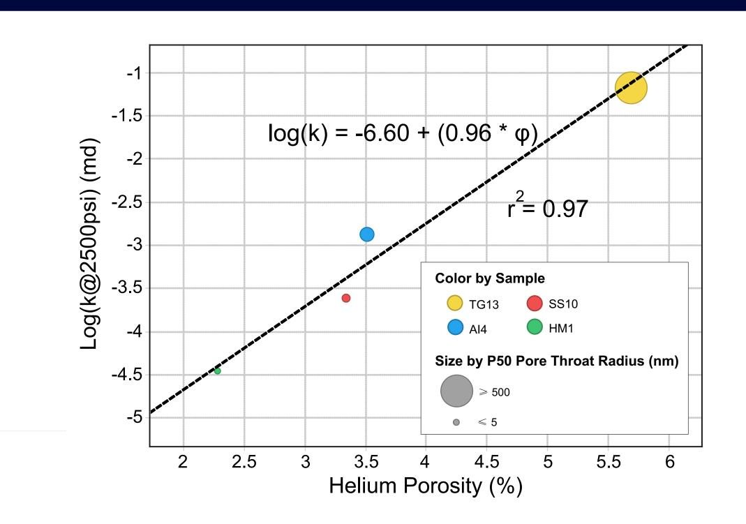
**Figure 10** - Helium pycnometry porosity versus log of permeability at 2,500 psi, illustrating the very good correlation observed between these two variables, as well as the dependency on the pore throat size
