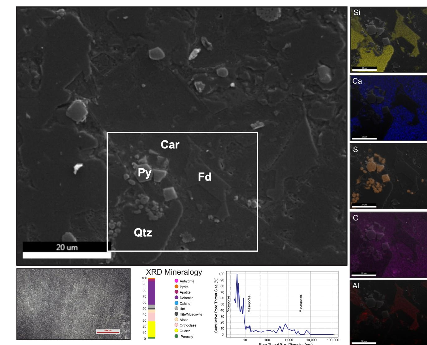
**Figure 14** - SEM image of carbonate-rich mudstone sample HM1 with associated elemental maps used in the identification of mineral phases, as well as sample photograph, XRD mineralogy and incremental pore size distribution curve from mercury injection
