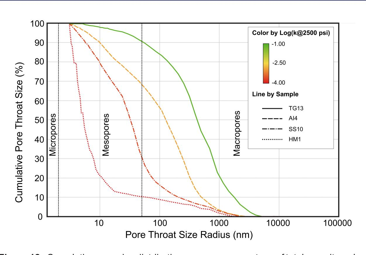
**Figure 12** - Cumulative pore size distribution curves as percentage of total porosity, colored by the log of permeability, for four samples with very distinct pore sizes bracketing the entire range of pore size distributions
