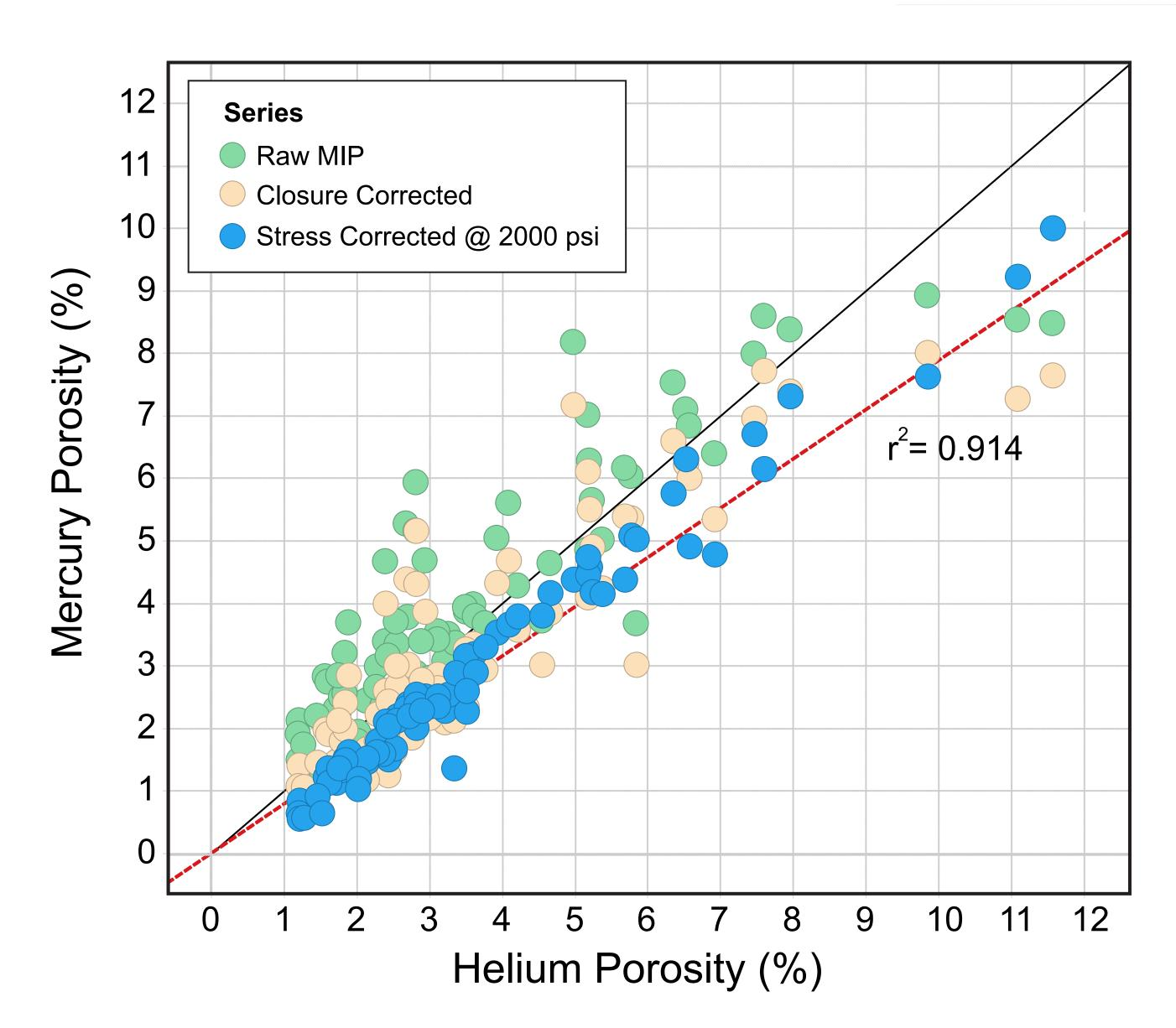
**Figure 9** - Crossplot of helium pycnometry porosity and the three different steps from mercury injection porosimetry (raw, closure corrected and net confining stress corrected), highlighting the greatly improved correlation between pycnometry and mercury injection once corrected, as well as the consistently lower porosity measured by mercury injection
