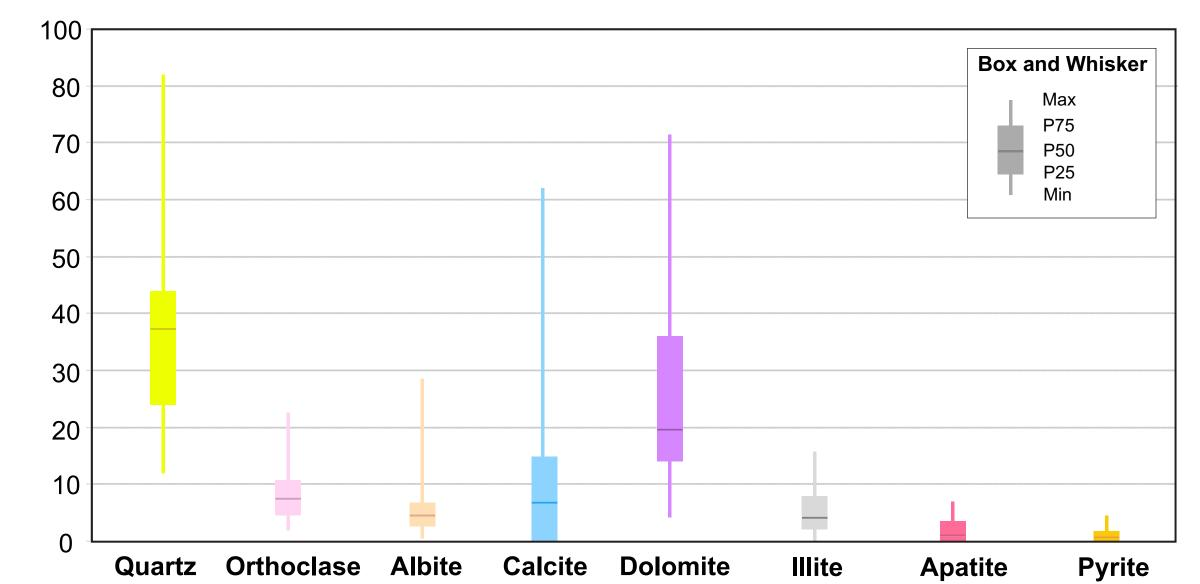
Figure 6 - Box and whisker plot of the main minerals present in the samples analyzed by XRD
