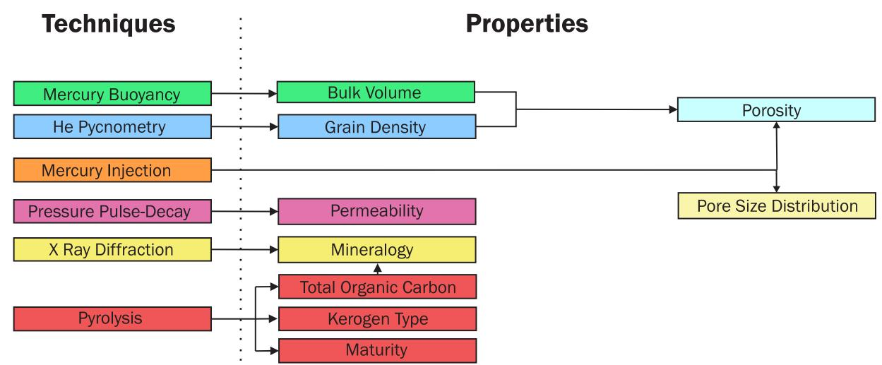
**Figure 4** - Flow chart of the methods used in this study in order to derive petrophysical and organic geochemical properties
