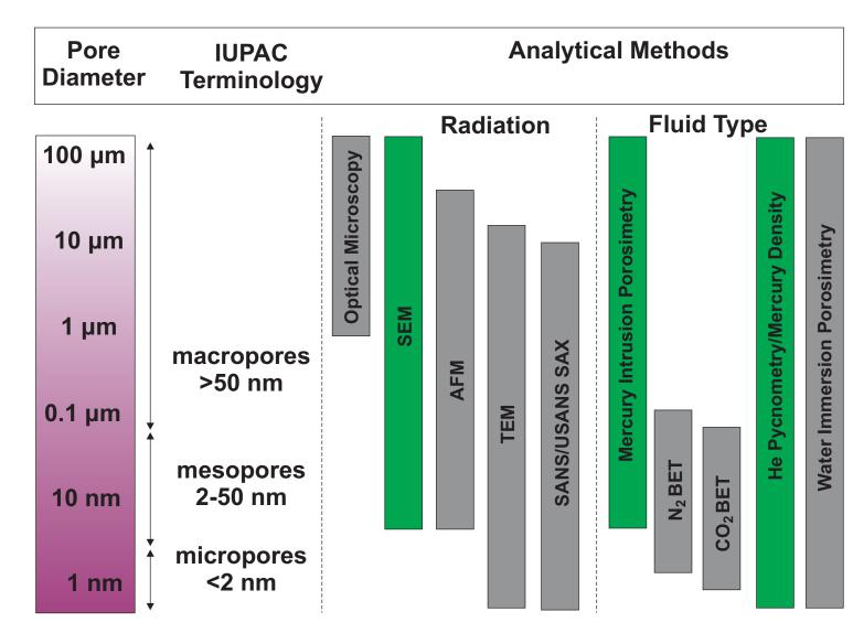
**Figure 5** - Analytical methods commonly used for determination of porosity and their ranges of pore size investigation, with methods used in this study highlighted in green
