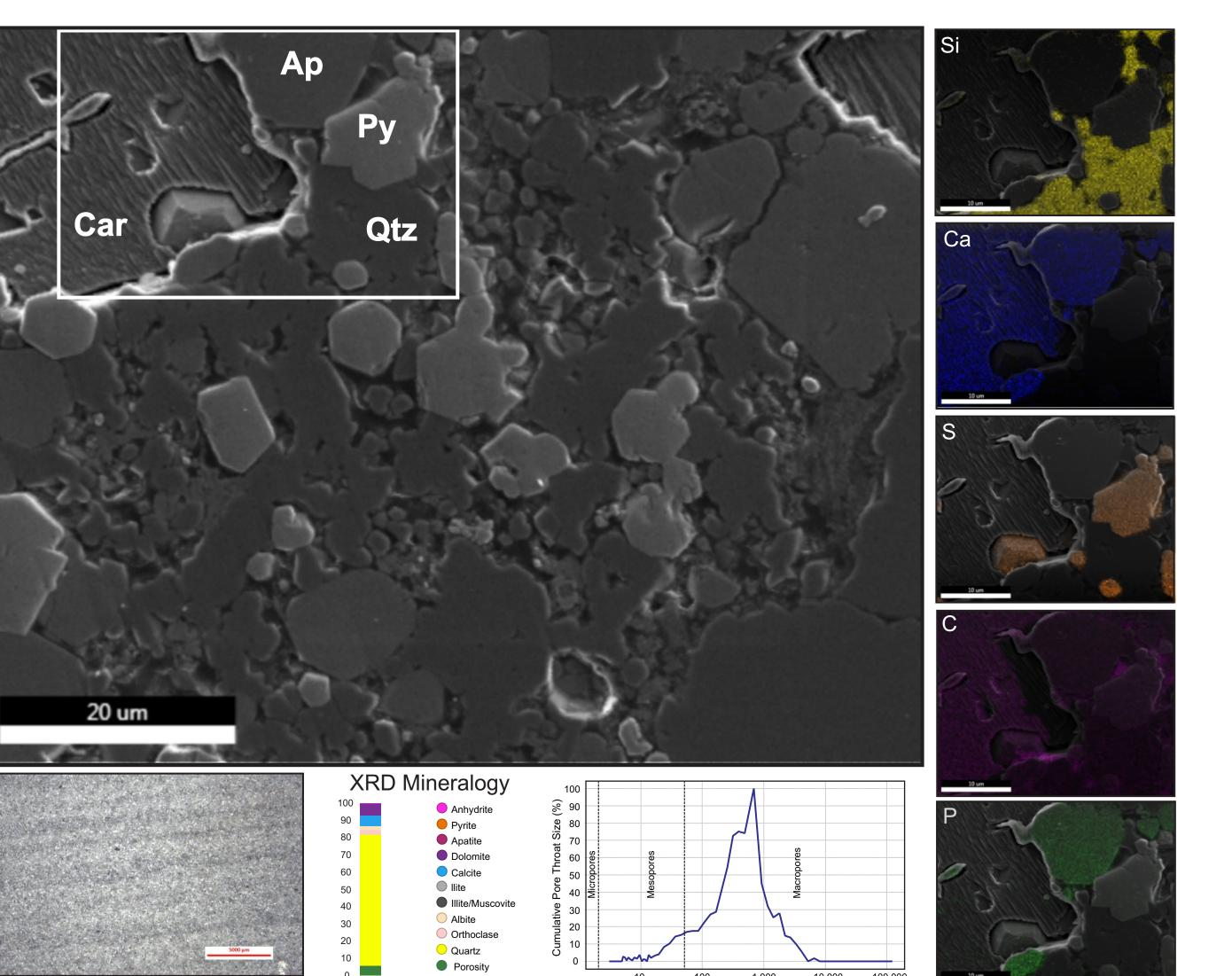
**Figure 13** - SEM image of silica-rich siltstone sample TG13, with associated elemental maps used in the identification of mineral phases, as well as sample photograph, XRD mineralogy and incremental pore size distribution curve from mercury injection
