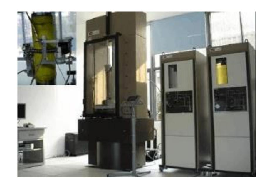
MTS815 electro hydraulic servo system
