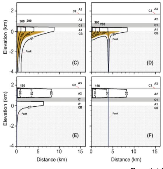
Even when faults are a significant distance from injection, basement faults could be perturbed
