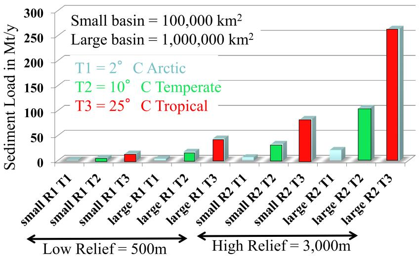
Tropical river basins can produce and transport 2.5 times more sediment than a similar scale basin located in a temperate region and 12 times more sediment than a similar scale Arctic basin
