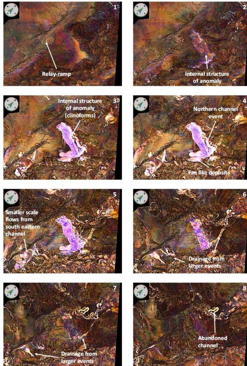
Figure 3. Iso-Proportional Slices from the NMF RGB blend through the anomaly, with 1 being the youngest and 8 the oldest. A number of events ranging from internal clinoforms, feeder channels and abandoned channels can be identified surrounding the anomaly.
