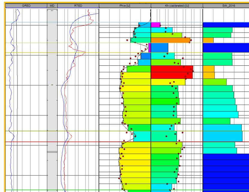
PC property assigned to Transverse section shows how the best RRT are being degraded from RRT1.
