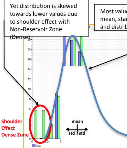
There are two important sources of porosity uncertainty. The first is related to logging tool measurement, processing and interpretation. The second is related to upscaling from logs to 3D model.
