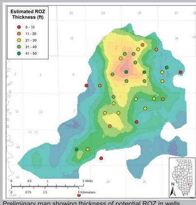
Preliminary map showing thickness of potential ROZ in wells in Noble Field based on petrophysical analysis overlain on an isopach of reservoir thickness. The ROZ, like the reservoir, is thickest at the crest of the structure.
