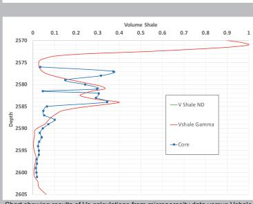
Chart showing results of Ve calculations from microporosity data versus Vshale calculations from wireline logs through an interval of the IVF. The lower section is clean sand and the upper portion is more heterolothic.
