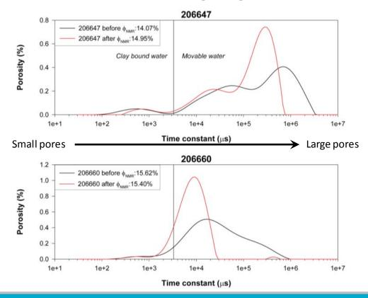
NMR T2 distributions in brinesaturated samples before and after core-flooding tests
