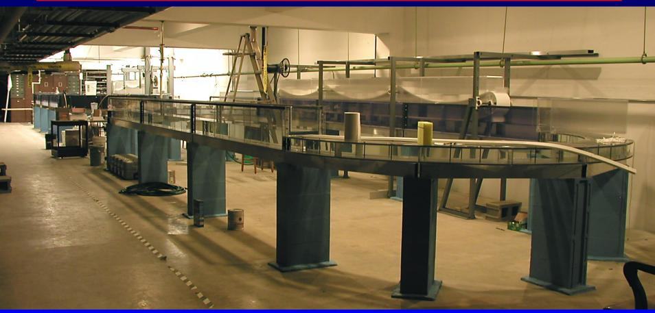
Racetrack design, 11 m long, 3 m wide, Flow Lid at 10 cm 25 cm channel width, 5 cm effective flow depth Paddle Belt instead of Centrifugal Pump **Floccule Friendly**
