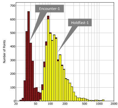
Difference in resistivity due to induction tools being run outside of Rt/Rm tolerance
