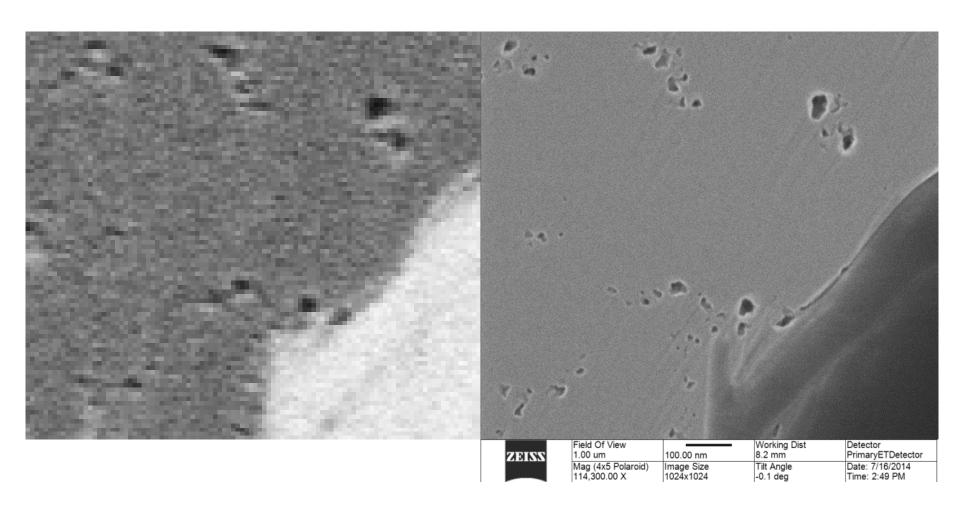
Much sharper definition of pore boundaries; linear pore at right is not detectable in SEM
