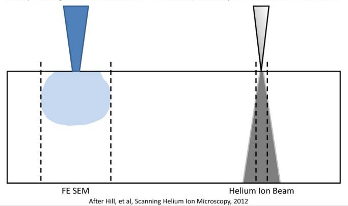
Presenter's notes: Helium ion beam secondary electron only (obviously primary beam is not electrons, can't have backscattered electrons).
