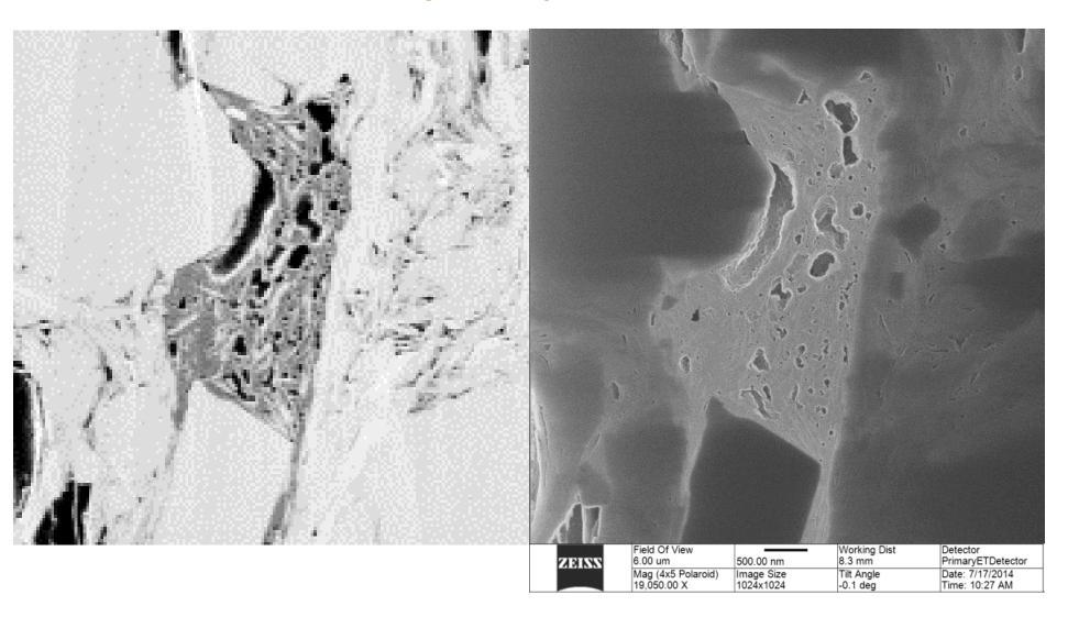
HIM image is effective at resolving small organic pores; less useful for imaging and calculating intergranular pores which are barely visible in image at right
