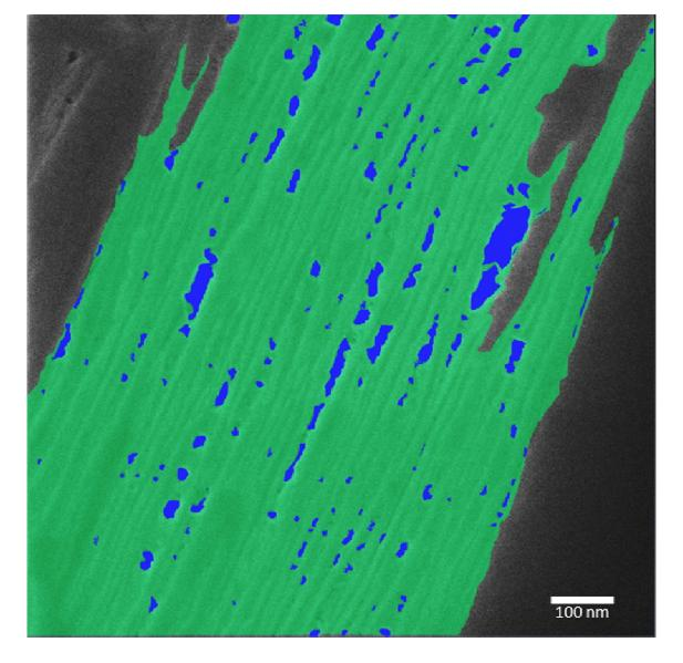
Segmentation result. Image pixel size is 0.97 nm. Green area represents boundary of clay particle; blue regions represent segmented porosity within clay particle. Total segmented porosity from this image is 4.71%.
