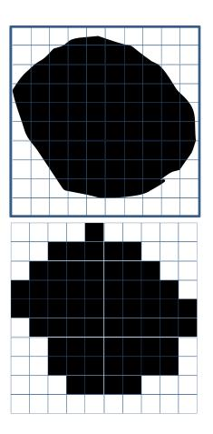
Sub 10-nm pore, HIM, 1 nm pixel size. 62/100 pixels classified as pore- 38% porosity reduction
