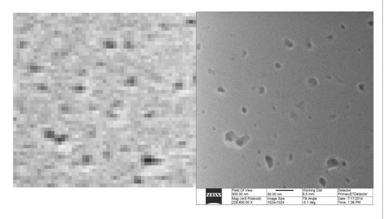
Extremely high resolution in HIM, pixel size below 0.5 nm. Smallest pore measured was 4 nm in diameter.
