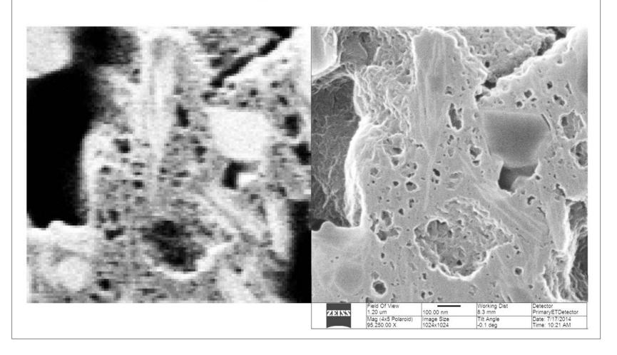
Presenter's notes: Higher energy of ion beam (larger particles) = ability to produce secondary electrons from surface at a different focal plane (inside pore).
