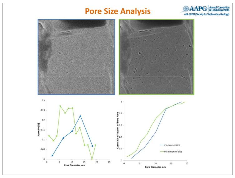
Presenter's notes: Quantifying ability to detect sub-resolution pores- left image 2 nm pixels, right image 0.8 nm pixels, pore size distribution confirms the increased segmentation of sub 10 nm diameter pores (4-5 pixels necessary for feature resolution).
