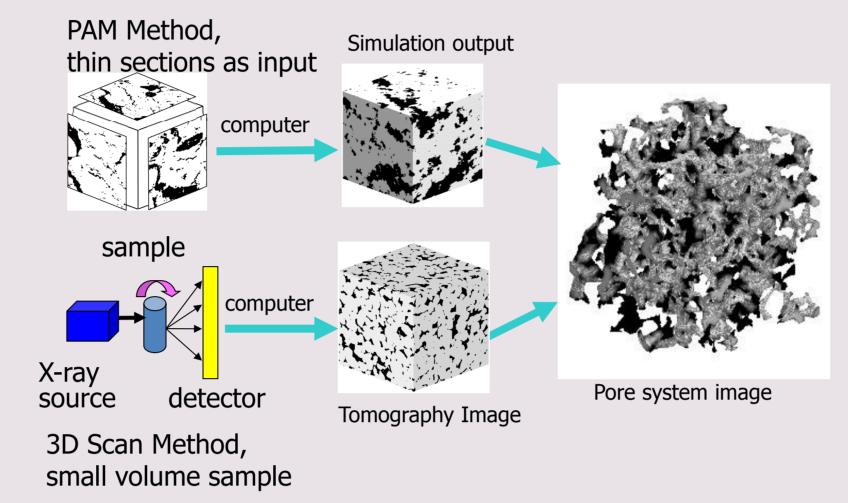
As an example of property estimation, the pore system can be used to calculate fluid flow. We can use multiple methods, but one that is useful is to derive a network model of the pore system, which retains both the geometric and topological characteristics in a reduced-dimension form.
