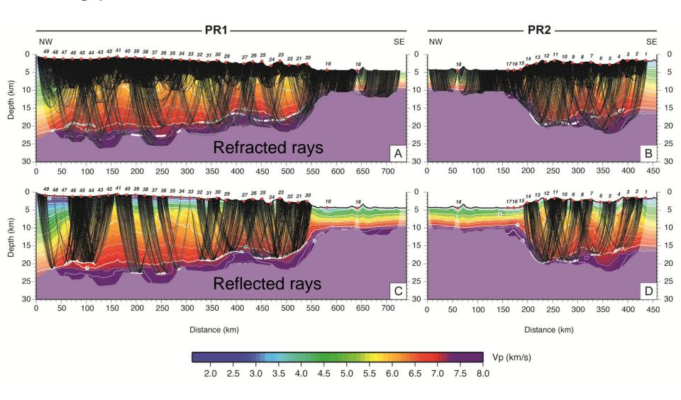
Modeling: joint reflection and refraction seismic travel time inversion
