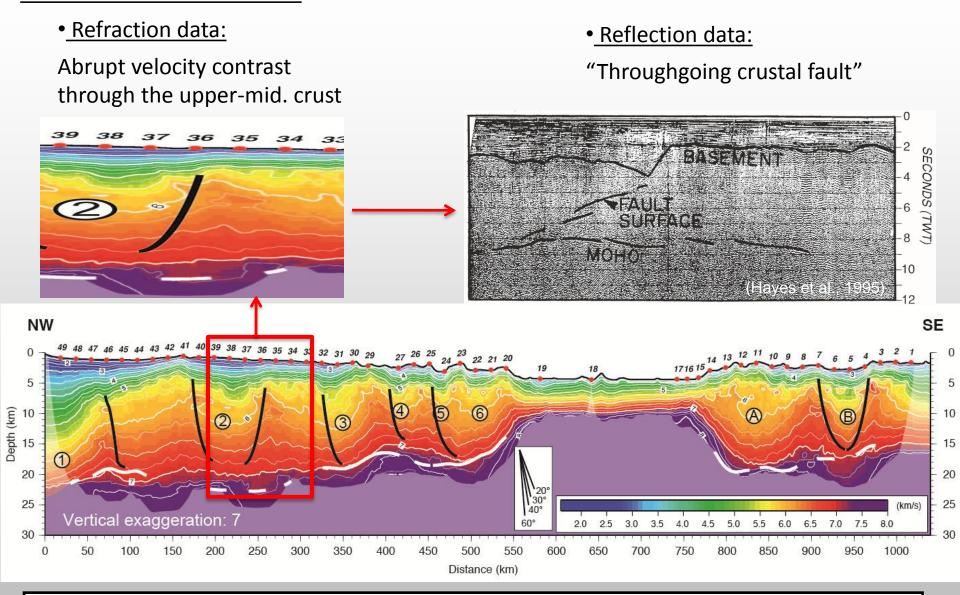
• Up. and Mid. crust = brittle deformation; Large-scale normal fault every 45-90 km
