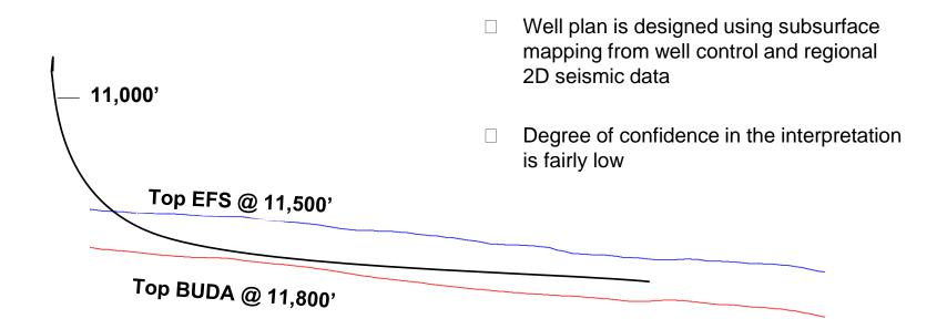
Target Line: 11578' TVD @ Zero Vertical Section Assuming Average 2 degree dip
