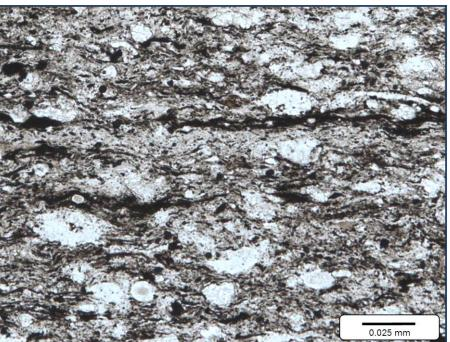
Standard 30 micron thick slide: No apparent grain support which would suggest poor reservoir quality
