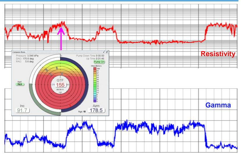
Azimuthal Resistivity Tool shows a visual image on a real-time Display (sees bed boundary ahead!)
