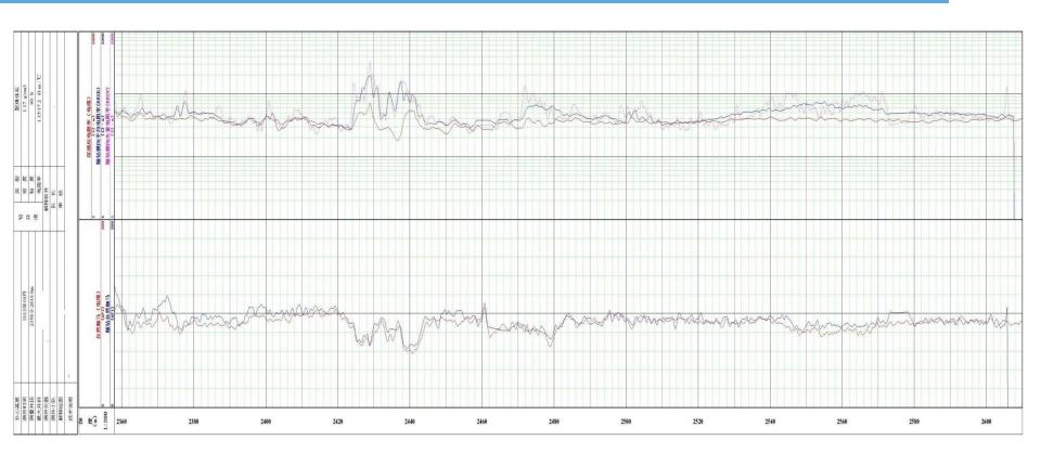
GRT resistivity compared with Dual Induction wireline tool. From 2424 - 2464 m. and 2520 - 2600 m. the ILD reads incorrect low resistivity. GRT works more accurately in thin horizontal beds
