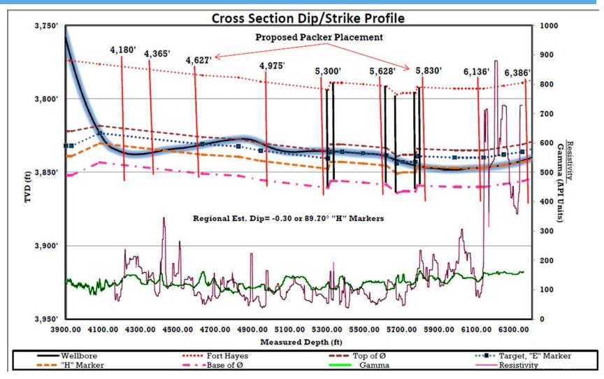
Borehole stayed in target zone for 98% of the well. Final 60 m fractured zone filled with oil.
