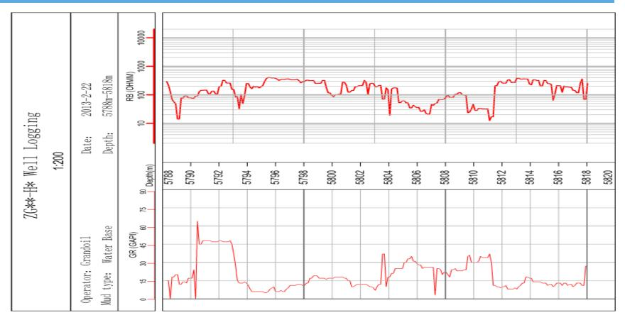
GRT was run in horizontal well that successfully completed and produced gas. The log shows the high-rate build section before the lateral was started.
