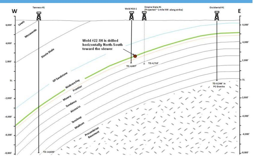
Niobrara shale is on top of a thin limestone target formation with 22° transverse dip-angle.
