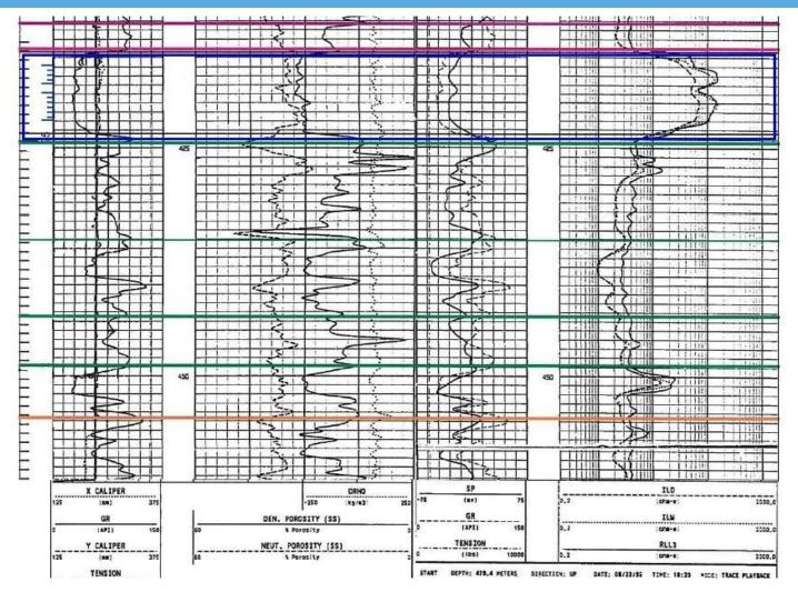
Target has 100 ohm.m. resistivity with good contrast to 3 ohm.m. upper and lower shales.
