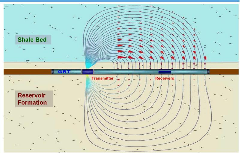
More current flows to upper receiver electrode, Indicating resistivity and direction of shale.
