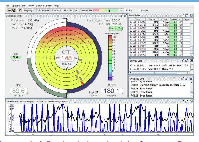
Color-coded Resistivity inside Compass-Rose image shows approach to overlying bed boundary
