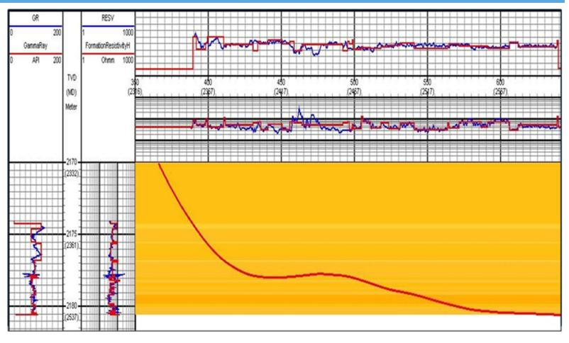
Total MD was 2983 m. with TVD of 2182 m. and lateral length 600 meters. GRT used to steer within the target formations for 188 hours.
