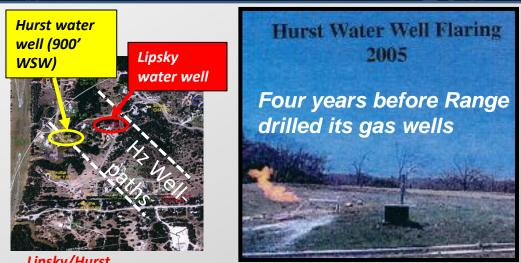
A water well inadvertently drilled into the Strawn in 2003 flowed 122,000 cf gas/day before it was P&A.
