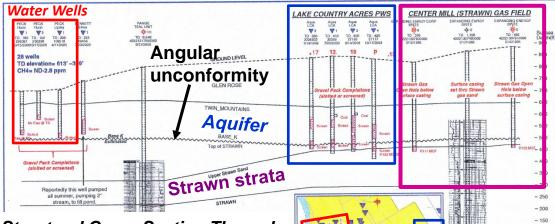
Structural Cross Section Through the Hurst and Lipsky Water Wells, the Teal Gas Well, Lake Country Acres Water Wells, and the Center Mill Gas Field
