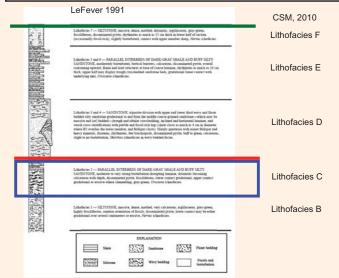
Middle Bakken lithofacies descriptions. Facies C is highlighted with a blue box. A sequence boundary (red line) separates faces C and faces D. A maximum flooding surface (green line) is identified at the top of the Middle Bakken. (from LaFever et al., 1991 and Sonnenberg, 2010)
