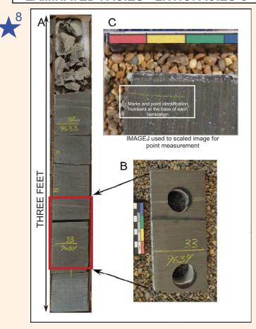
Core section (A) shows location of core photo (B) of facies C from Liberty 2-11H - laminated, argillaceous, calcareous siltstone/sandstone.
