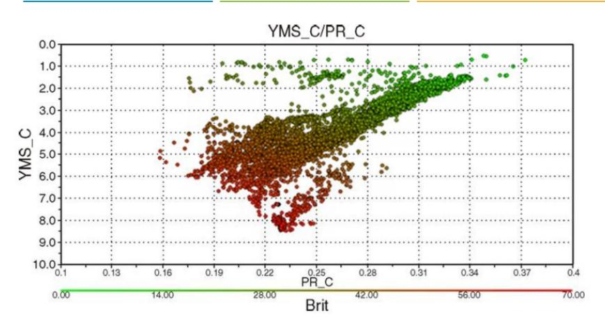
Next, let's discuss how to determine geomechanical properties. The figure above, from Rickman et al. (2008) crossplots static Young's modulus (YMS) vs static Poisson's ratio (PR) and calibrates the result to brittleness (Brit).
