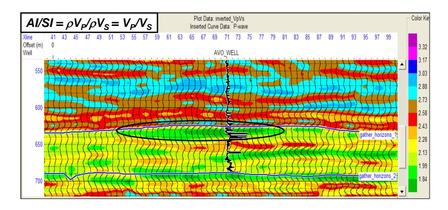
Here is the ratio of *P* to *S* impedance, which is equal to the ratio of *P* to *S* velocity. Notice the low ratio at the gas sand.
