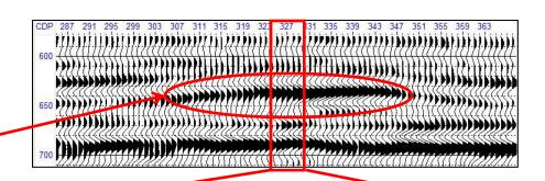
The seismic line is the "stack" of a series of CMP gathers, as shown here.
