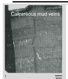
Veins form during sediment dewatering, initiated by diatom frustule collapse during compaction and by overloading during downslope slumping
