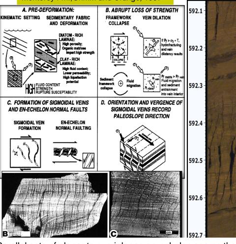
Parallel sets of planar to curviplanar, en-echelon seams that bifurcate into distributary networks. Various terms include: tension gash arrays, veins, stratal disruption, spaced foliation, kink bands, crenulation folds, web structures, cataclastic fabrics, scaly foliation, web structure and microstructural domains
