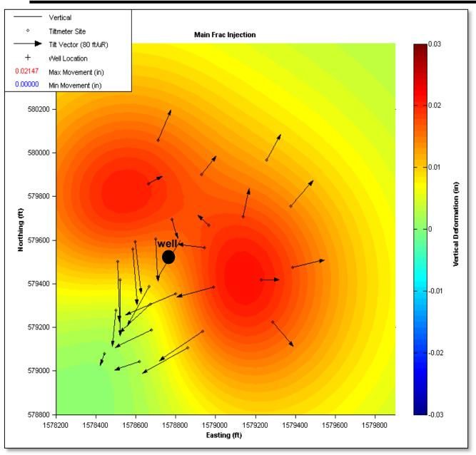
Surface tiltmeter mapping measures the fracture induced tilt at points above a hydraulic fracture and then solves the geophysical inverse problem to determine the fracture parameters that produced the observed deformation field.
