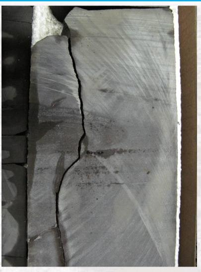
Soft sediment deformation slump within thin interbedded grainstone and organic rich siltstone laminations (UV on left, WL on right). Gil B. suggested I may have a new giant fusulinid, *Gigantuana species*?
