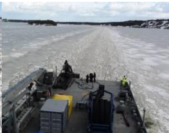
The SYKE oil combat module: Can be built in 6 m brush width, securing a 24 m wide sweeping area
