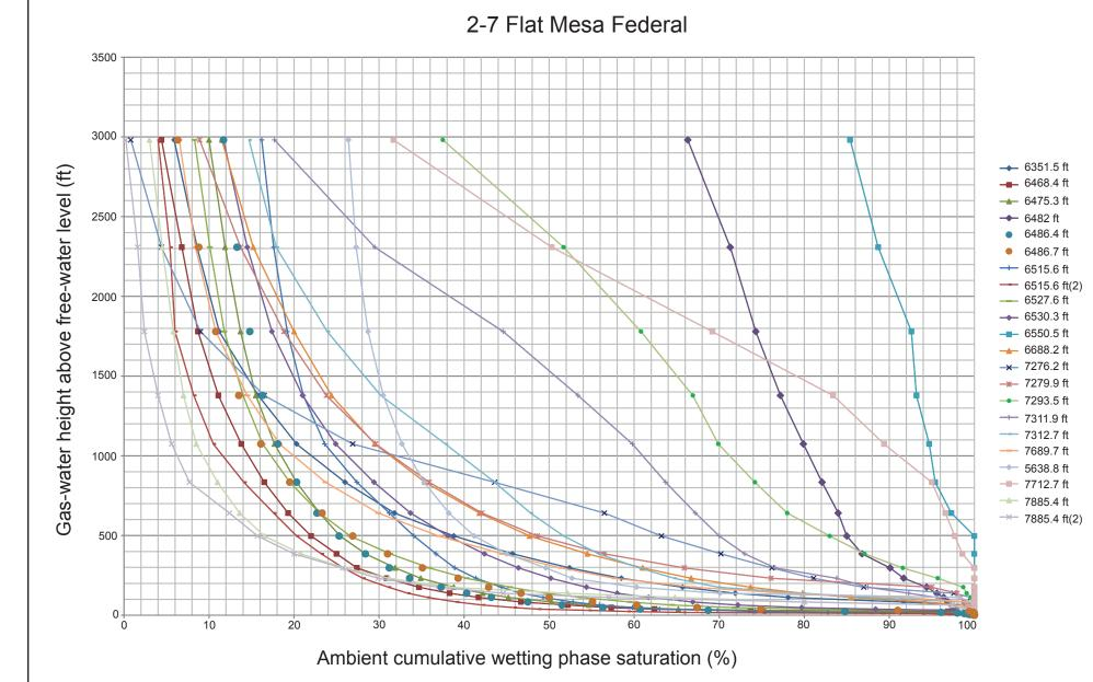
he graph shows data for the well 2-7 Flat Mesa Federal. The data were provided by Byrnes nd Cluff (2009) and include -brine capillary pressure data for 21 samples. The curves ally present asymptotic reducible water saturations Swirr) around 10% to 30% which are usually higher than the log derived (Buckles plot)
