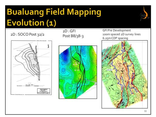
Presenter's notes: This sequence of illustrations shows the evolution of the field mapping--how the structure mapped changed with each vintage of seismic and post-drilling. The trap area, described by the oil-water contact at -1130m tvdss, is approximately 2145 acres (8.7 square km). There is a possibility that the field may be extended into the undrilled fault block to the east (the "eastern terrace" prospect). SEL is scheduled to drill step-out well in the near future.
