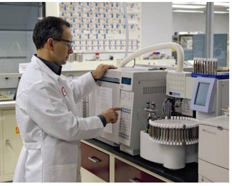
Analysis of samples by automated thermal desorption/ gas chromatography/mass selective detection
