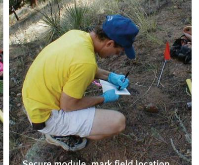
Surface geochemical sample acquisition in the soil zone. Samples left in residence for ~20 days, for the equilibration of adsorbents to in situ organic compound signature
