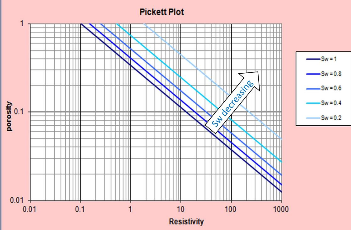
**AND**: Bulk volume water, BVW = Phi \* Sw BVWminimum implies Sw irreducible, which implies little or no water production.
