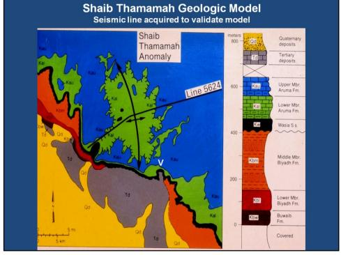
Presenter's notes: Shaib Thamamah map showing seismic line 5624 that Saudi Aramco acquired to test the geologic model.
