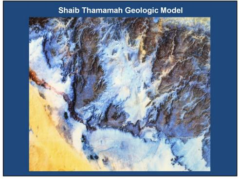
Presenter's notes: Shaib Thamamah anomaly. Gently NE-dipping Upper Member of Aruma Fm. (dark signature) is warped into a structural terrace that is eroded to expose the Lower Member (bright signature).
