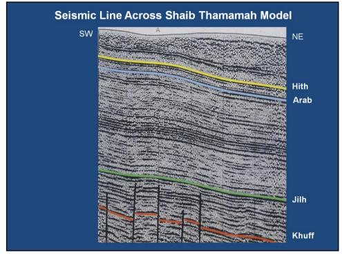
Presenter's notes: Line 5624 across S T anomaly. Regional NE dip is interrupted by structural terrace overlying basement faults. The five faults account for the large extent of the anomaly.
