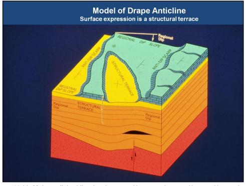
Presenter's notes: Model of fault-controlled anticlines that migrate upward into structural terraces with geomorphic expression.
