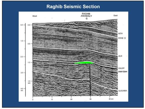
Presenter's notes: Seismic line 4134 across Raghib field which is a drape anticline above a basement fault. Oil from the Qusaiba (Silurian) source rock migrated up the fault and was trapped in the Unayzah Sandstone (Permian), which is sealed by the impermeable Khuff Limestone (Permian).
