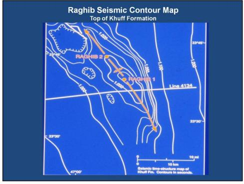
Presenter's notes: Seismic contours (seconds) on top of Khuff Limestone that overlies the Unayzah reservoir sandstone.
