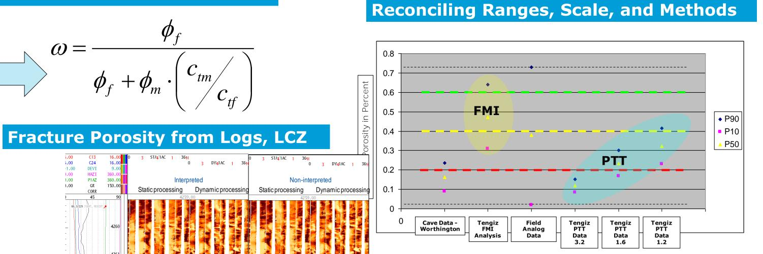
ge of estimates of fracture porosity: cave maps, FMI logs, dual porosity PTT. PTT offers much ger scale than logs, and dynamically sensed volume as prosed to statically measured volume.
