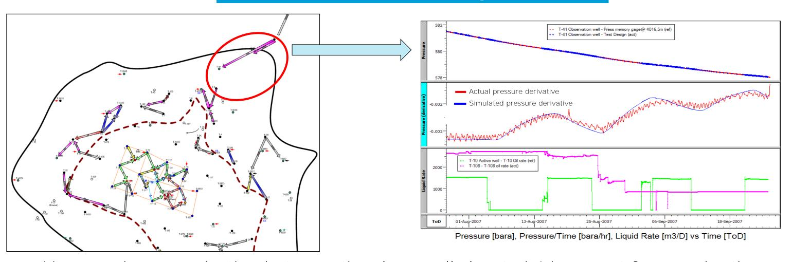
Very good communication between the slope wells located 4 km apart from each other and completed in different stratigraphic intervals. Pulse tests also support fracture directions - higher diffusivity parallel to slope than perpendicular to slope
