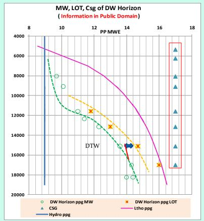
The Narrow DTW in addition to the presence of hydrocarbon led to serious drilling challenges
