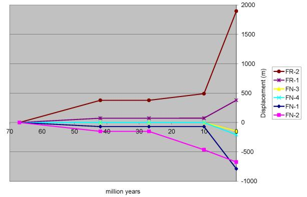
• Strain analysis proves it is a linked system, normal and reverse faults mirror each other in both timing and strain (net compression = net extension).
