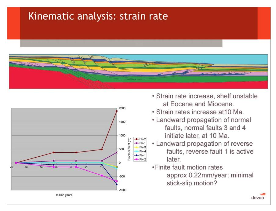
Notes by Presenter: Plotting displacement through time for each fault, allows us to understand deformation ratio, stress partitioning, and linkage of the system.
