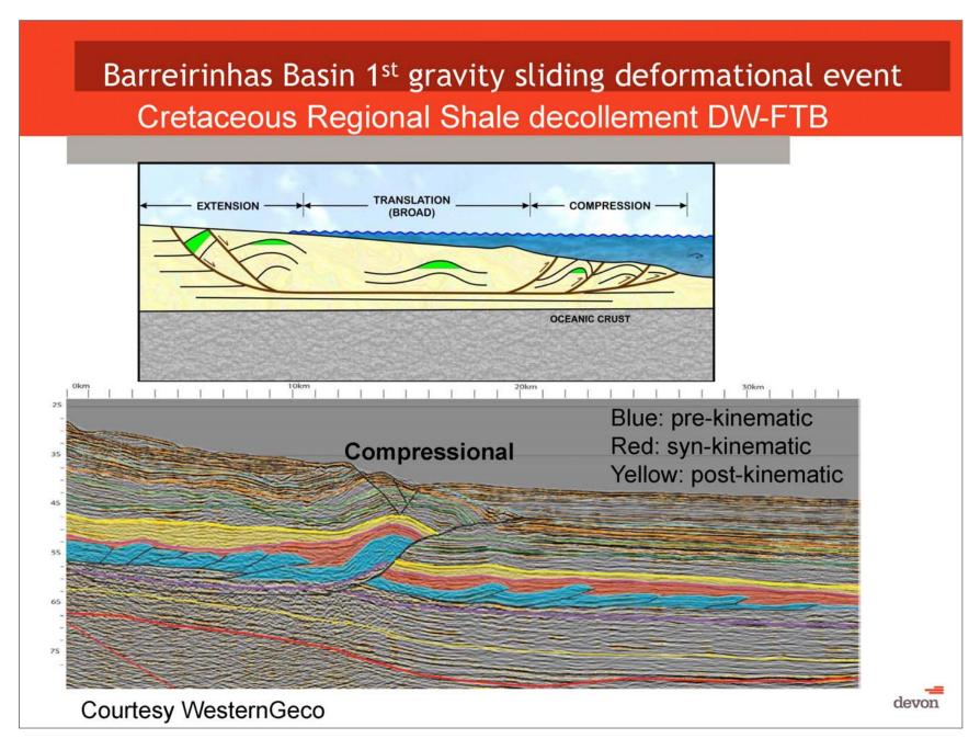
Notes by Presenter: This is a detail on the compressional domain of the Cretaceous system. In Blue is the pre-kinematic (pre-Phase 1) sequence Note crosscutting by Phase 2
