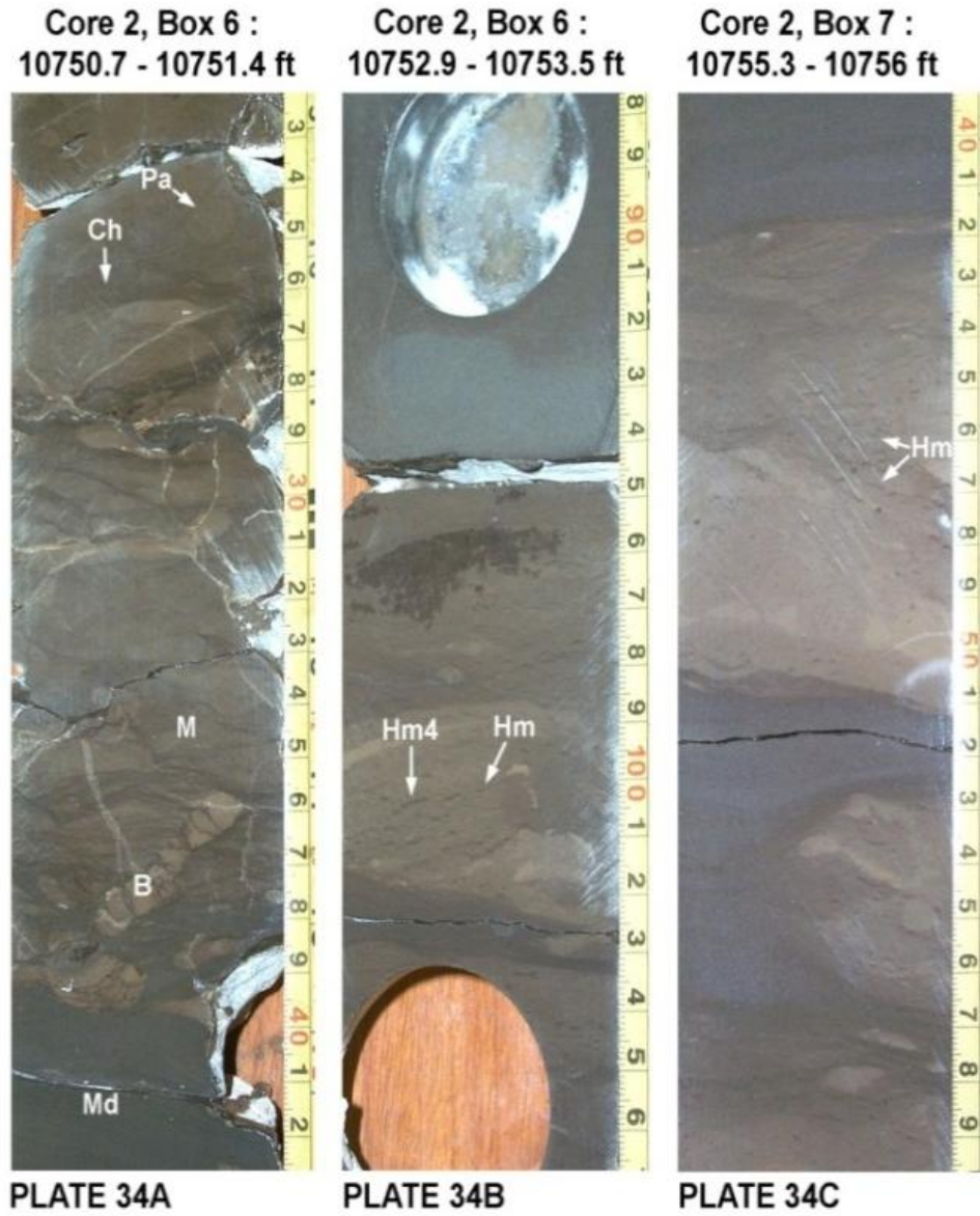
Figure 6. Core showing bioturbated lime mudstones and wackestones interbedded with slightly dolomitic argillaceous lime mudstones in MN-138. Lower Makhul interpreted as middle ramp.
