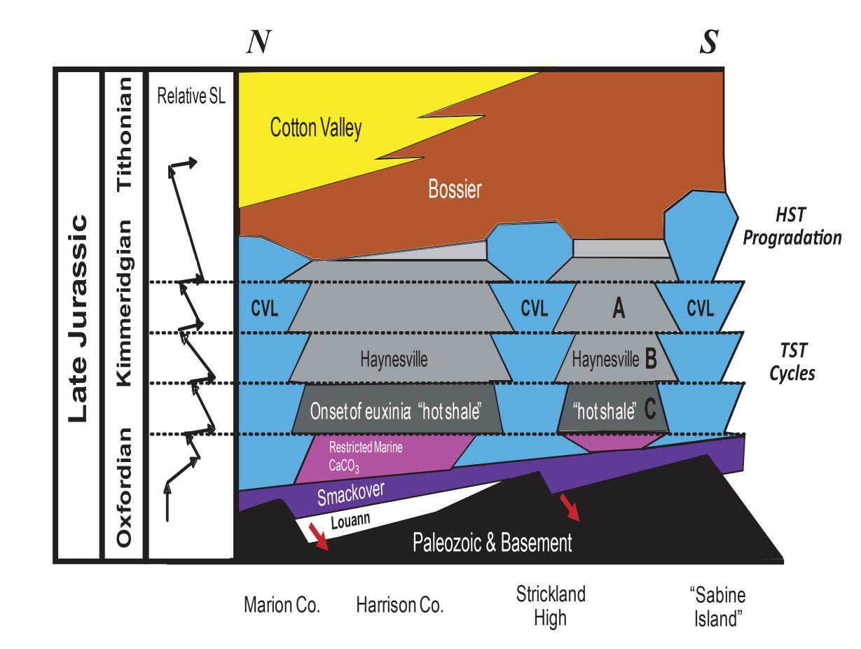
Schematic N-S cross section of Haynesville Shale depositional system in the Texas and Louisiana play area. Units labelled A, B, and C ("hot shale") constitute the shaley, organic-rich facies of the Haynesville Formation.
