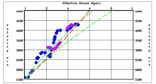
Velocity to effective stress calibration using a hybrid model (red curve) that moves from the minimum fluid pressure model at low effective stress to the maximum fluid pressure model at high effective stress.
