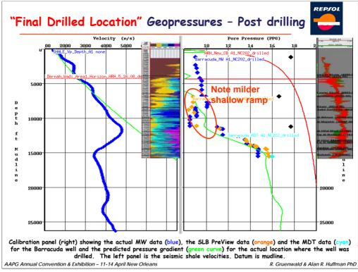
*Presenter's Notes:* This is the velocity function from the actual drilled location, which is 250 meters from the original prediction location. Note the decreased shallow ramp behavior. This velocity function predicts a lower pressure at 9,000 to 10,000 feet than the original location. Green curve on right with half ppg error bar final location prediction
