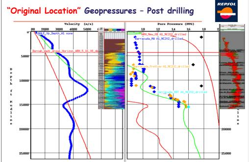
Calibration panel (right) showing the actual MW data (blue), the SLB PreView data (orange) and the MDT data (cyan) for the well and the original predicted pressure gradient (green curve). The left panel is the seismic shale velocities. These are for the original predicted location. Datum is mudline.
