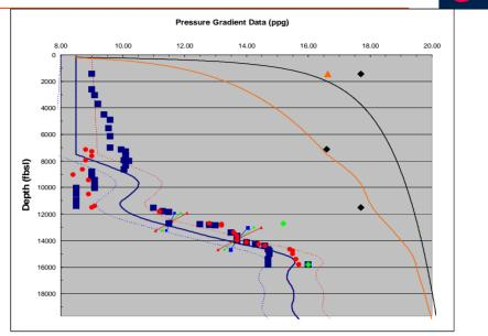
Pre-Drill Prognosis with drilled under / over pressure ramp
