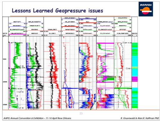
**Presenter's Notes:** The well did not kick at the 12772' MDT point because it is likely laterally connected to a reservoir "isolated centroid", or connected by fracture deeper part of the reservoir like a short circuit but disconnected from shale behavior
