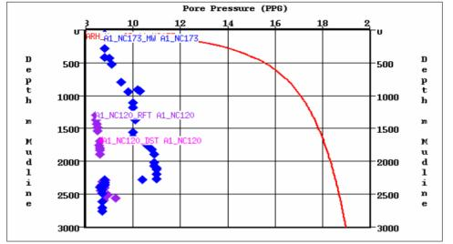
Offset pressure data from the NC 120-A1 (purple and magenta) and NC 173-A1 (blue) wells that had seismic data support
