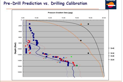
Original prediction from pre-drill location with actual drilling data including drilled MW (blue), PreView data (red) and MDT data (green). The MDT at 12,772' is likely to be supercharged (SLB final)
