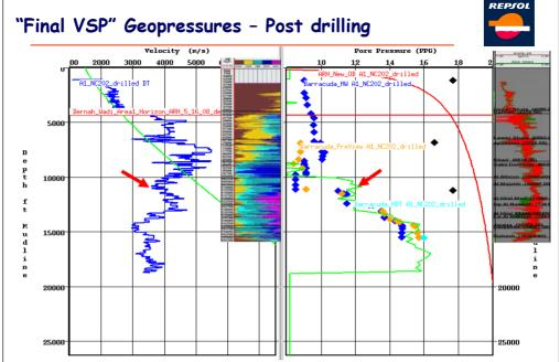
Calibration panel (right) showing the actual MW data (blue), the SLB PreView data (orange) and the MDT data (cyan) for the well and the predicted pressure gradient (green curve). The left panel is the Vp from the VSP inversion. The minima on the sonic curve are the shaley zones. Datum is mudline.
