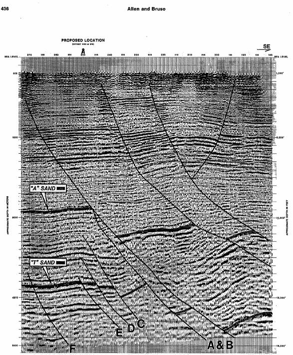
Fig. 10. Depth section constructed from smoothed stacking velocities shown in Figure 9. Notice the reversal in seismic dip at the A sand and deeper between shotpoints 260–245 as compared to dip on Figures 3 and 7. The proposed location is shown at shotpoint 250.
