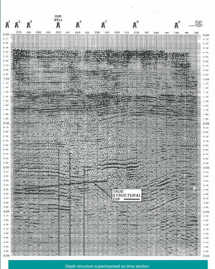
Note the vertical alignment of horizon breaks. From Allen and Bruso. 1989
