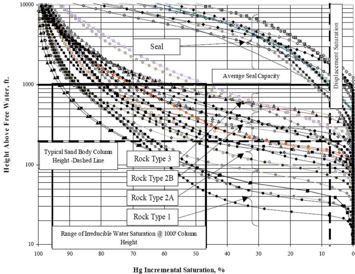
Figure 11. High pressure, mercury injection capillary pressure data converted to height above free water level. Note that the range of initial water saturation at 200 ft of column height is 30%-100%. It takes 1000 ft-2000 ft of column height to have water saturation in the measured range of 5%-40%.
