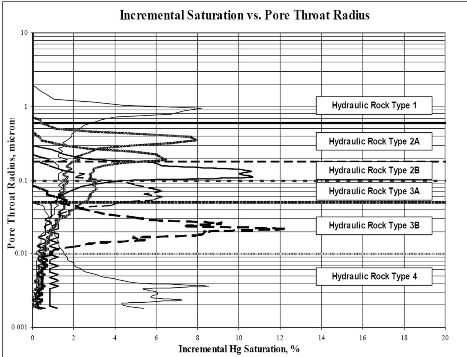
Figure 6. Incremental mercury intrusion plot used to identify hydraulic rock types for the Bossier sands.
