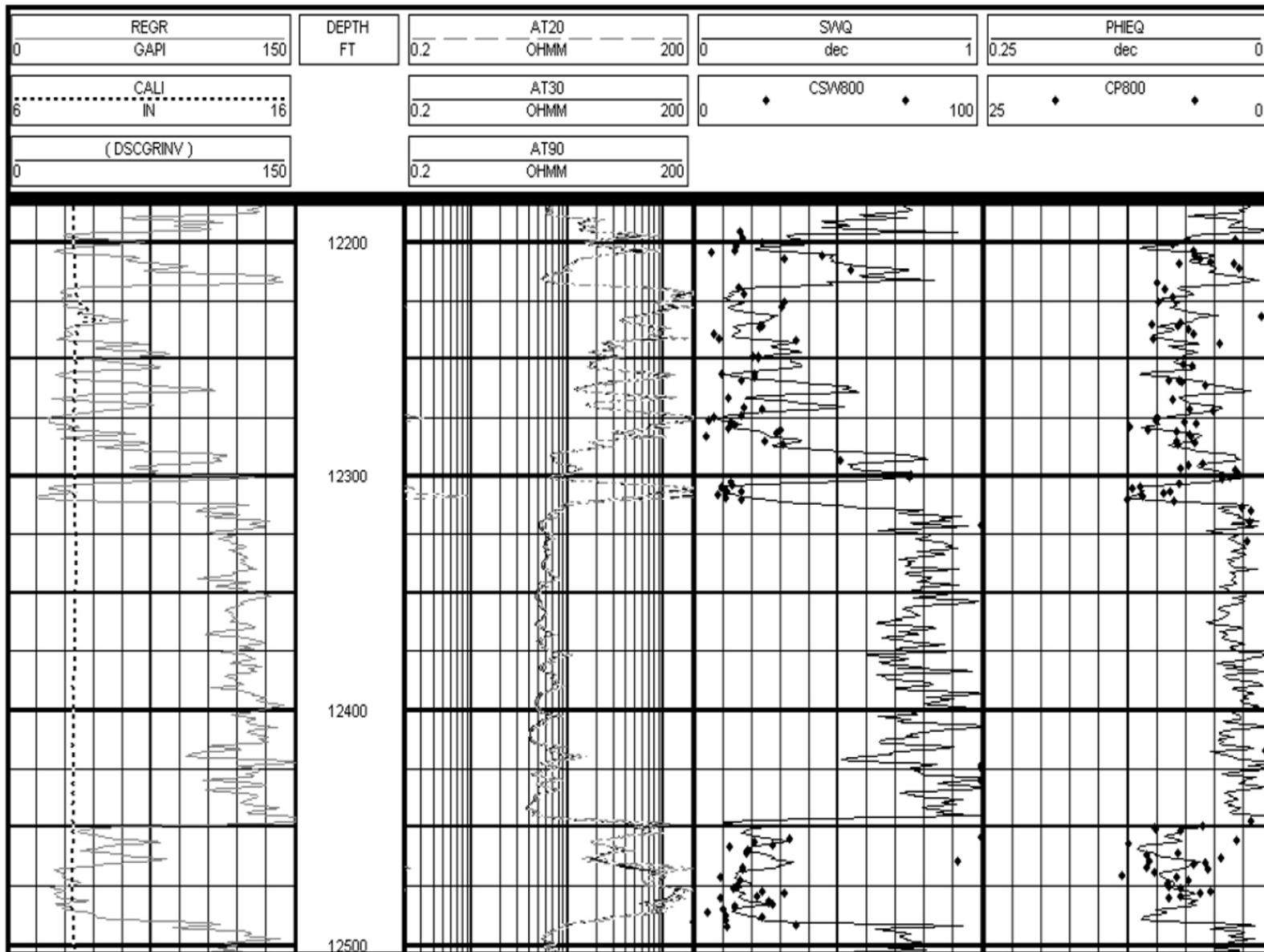
Figure 10. Log profile of gamma ray (track 1), resistivity (track 2), water saturation (track 3), and porosity (track 4). The discrete points represent the measured water saturation and porosity from the core. Note that there is close agreement between the core and log values for both water saturation and porosity.
