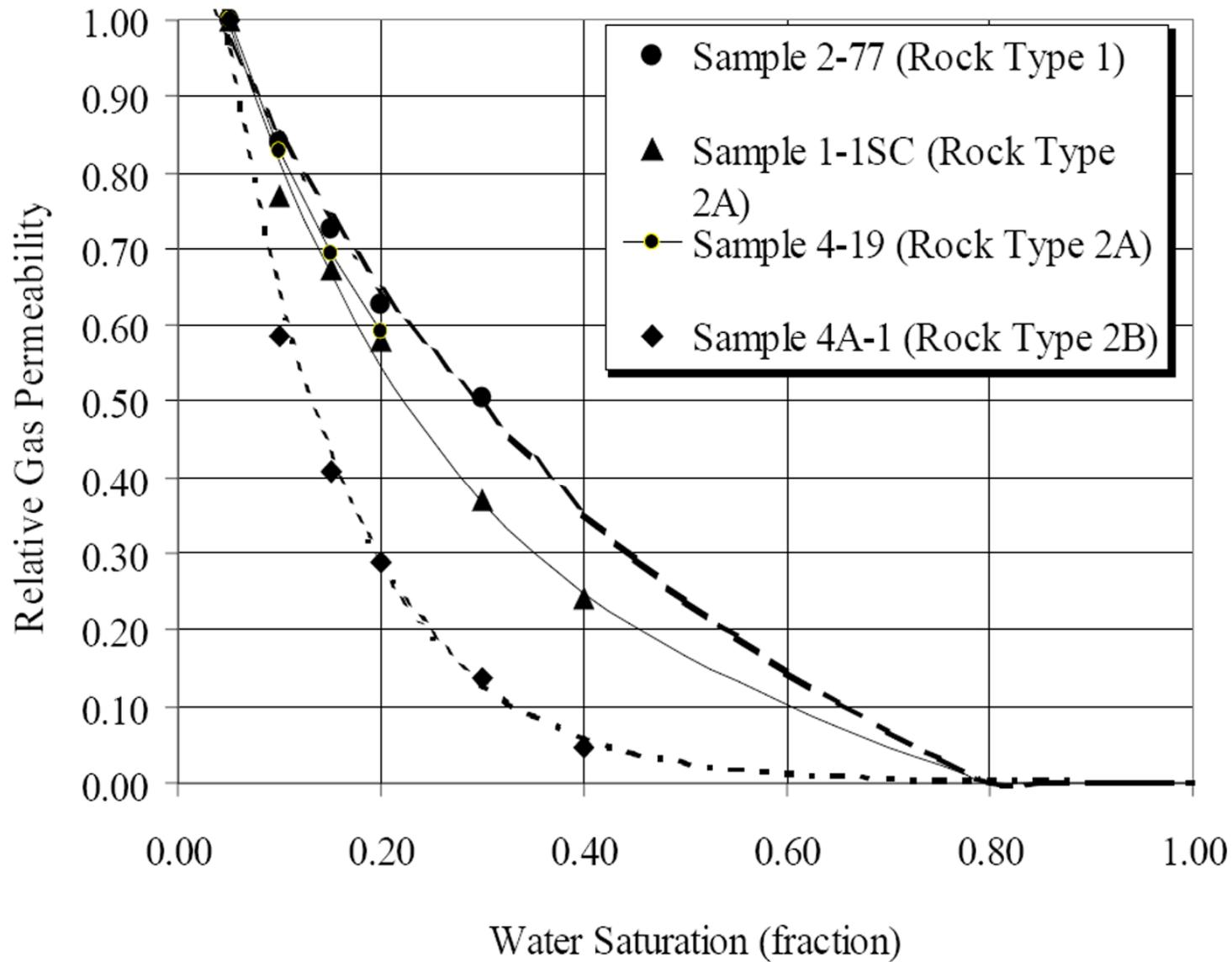
Figure 8. Relative permeability curves for hydraulic rock types 1, 2A and 2B. All curves were normalized to 5% initial water saturation based on the minimum water saturation measured in rock type 1.
