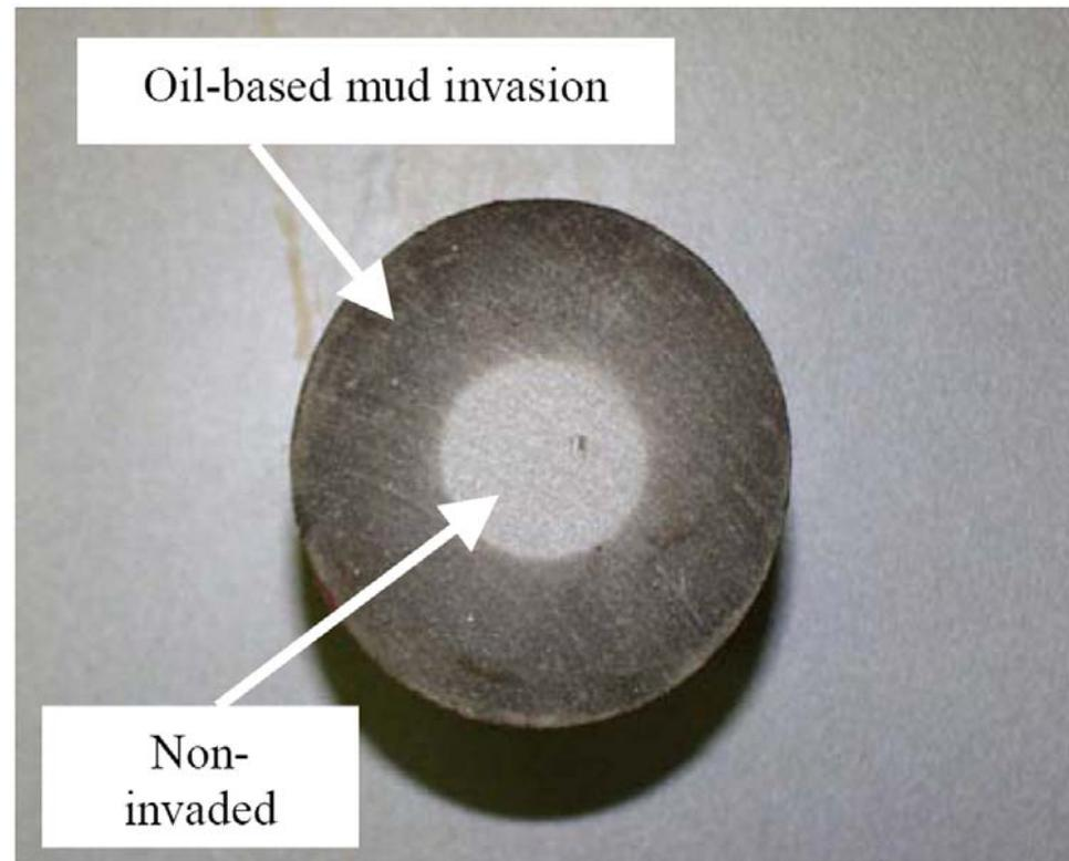
Figure 9. Photograph of a whole core section illustrating oil-based mud invasion profile in one of the most permeable rocks (i.e., hydraulic rock type 1). Note, however, we still observe an undisturbed portion of the core.
