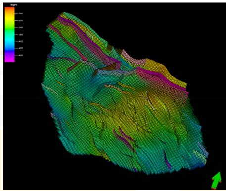
Faults imported into the VISAGE Geomechanical model.
