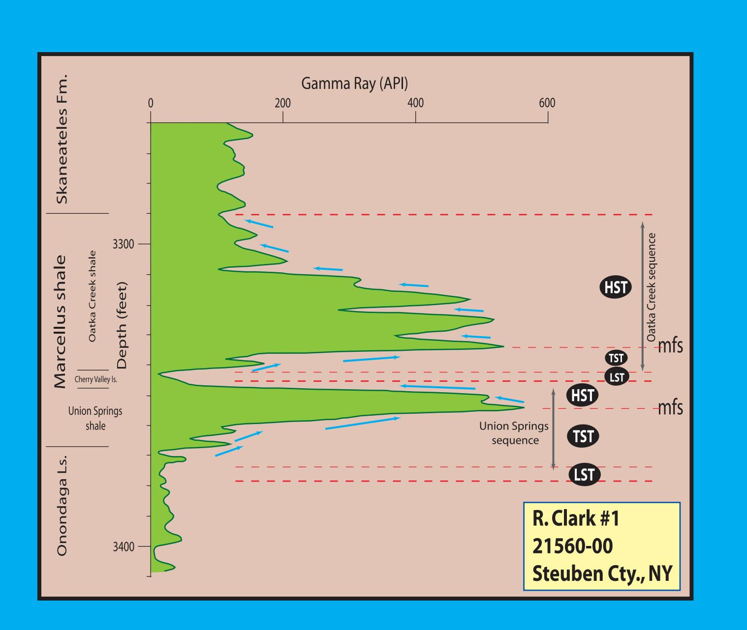
Parasequence (fourth order depositional sequences) stacking arrangement in the Union Springs and Oatka Creek shale members of the Marcellus Shale. The two Marcellus depositional sequences span ~1.5 MY (blue arrows denote the inferred fourth order cycles; arrows pointing to the right imply a landward shift of environments; arrows pointing to the left imply an offshore shift of
