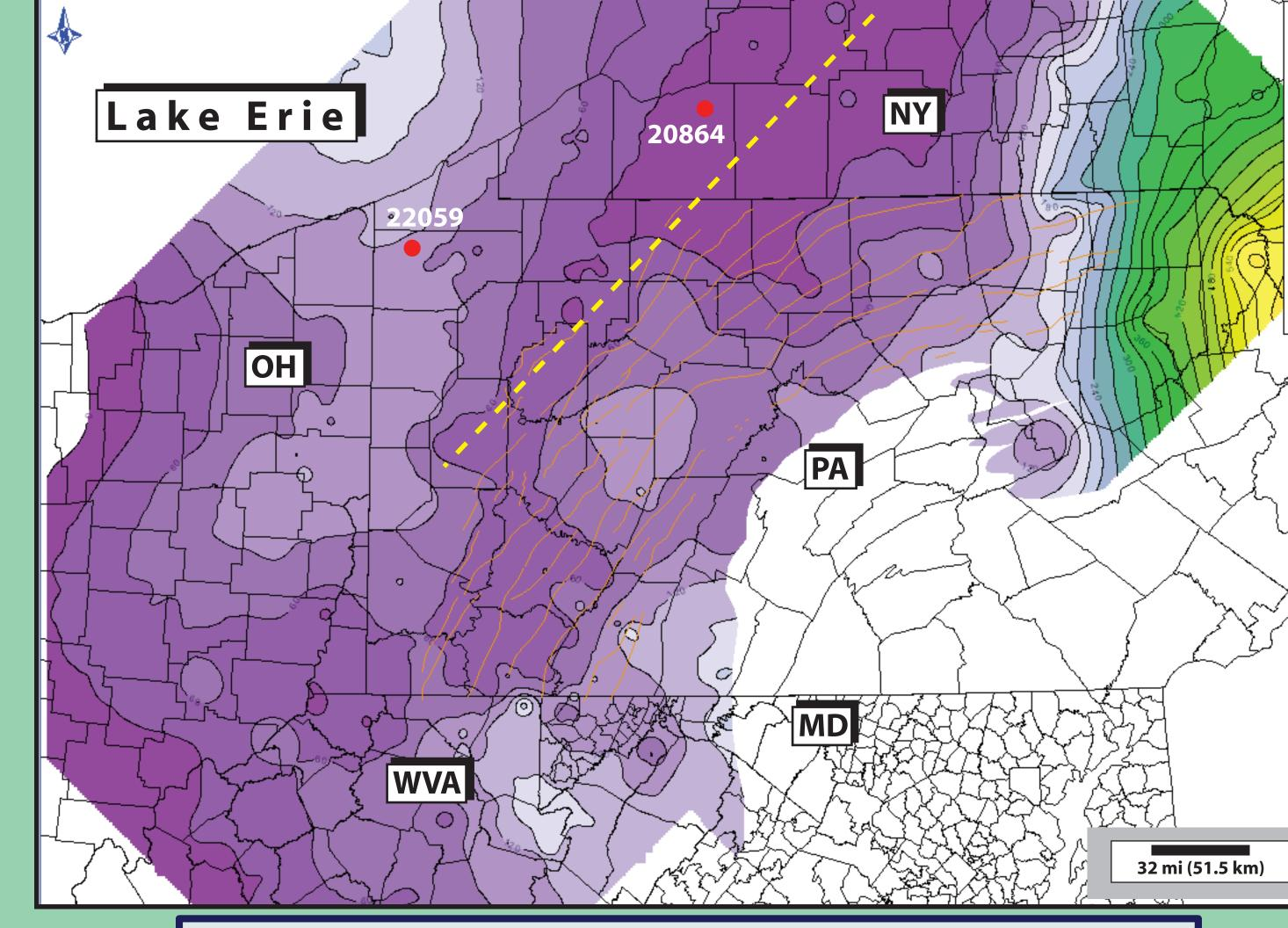
Isopach map of the Oatka Creek Shale (thickness in feet), the upper unit of the Marcellus Shale. The red circles denote the locations of wells 22059 and 20864; note the thinning of the Oatka Creek Shale to the east and west of the axis of thinning (dashed yellow line).
