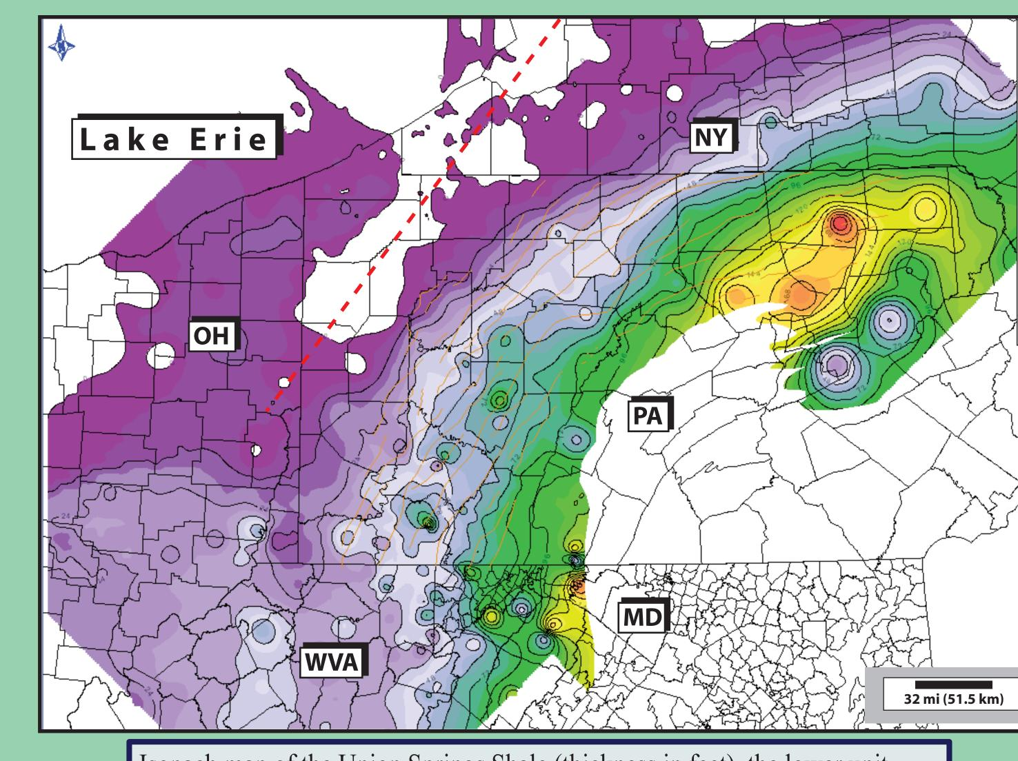
Isopach map of the Union Springs Shale (thickness in feet), the lower unit of the Marcellus Shale; dashed red line denotes the axis of minimum thickness of the Marcellus in the western New York - northwestern Pennsylavania region of the basin.
