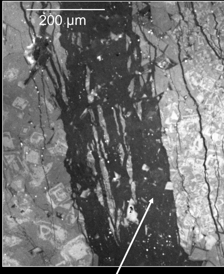
Crack-seal in synkinematic cement
