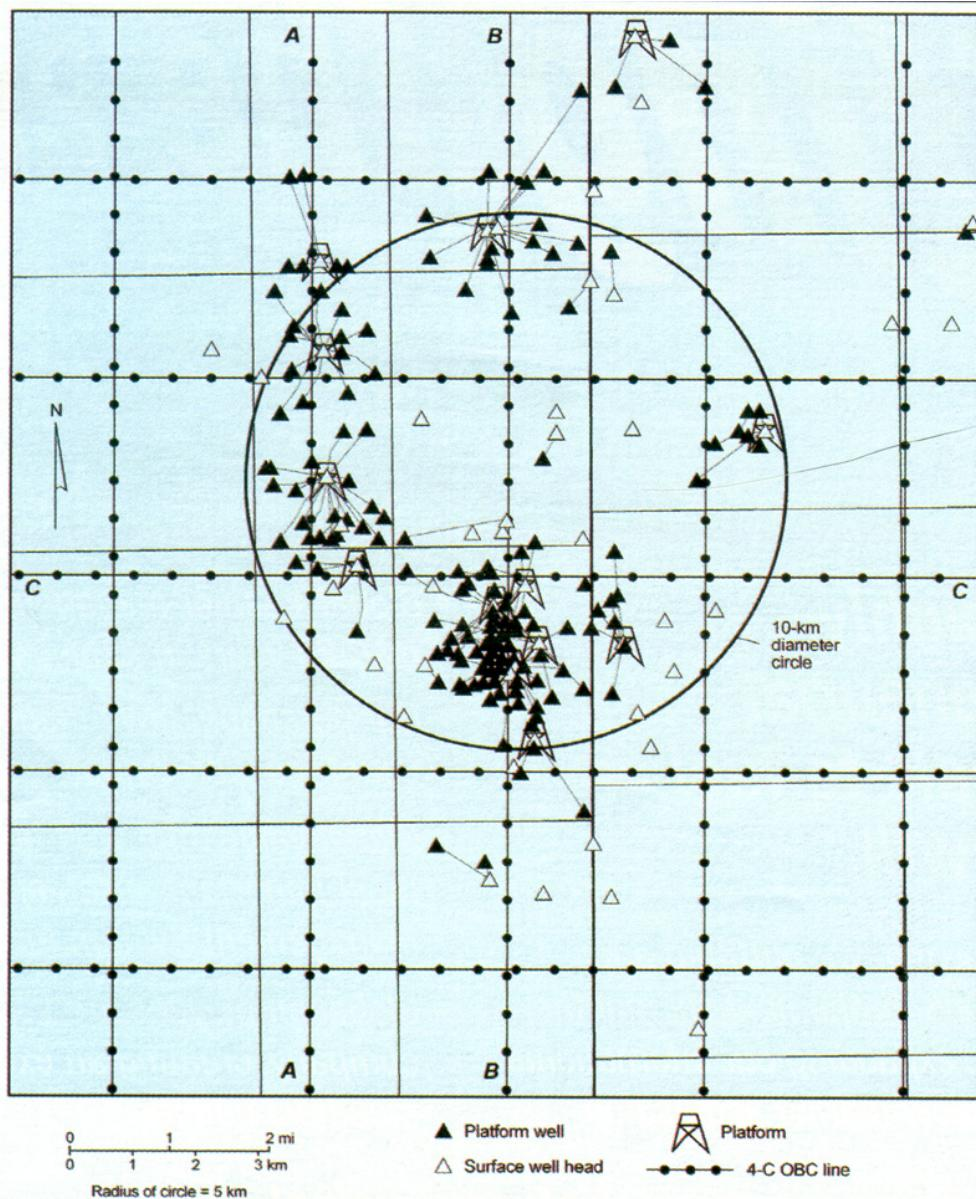
**Figure 2.** 4-C OBS data acquisition across one specific area of production congestion. Note how close OBS lines AA, BB, and CC are to many of the production facilities.
