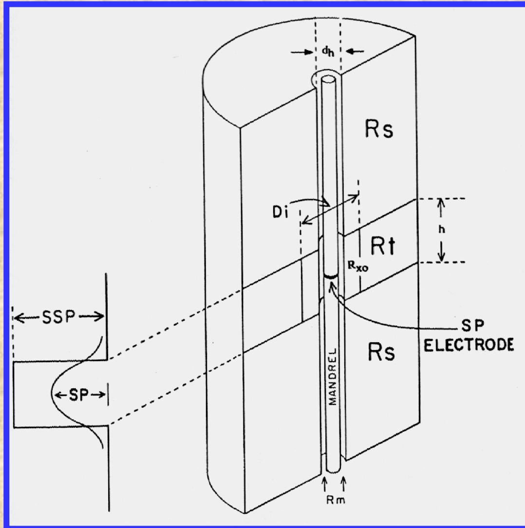
SP is heavily affected by bed thickness ( $h$ ), and by the ratio of  $R_t/R_{mud}$
