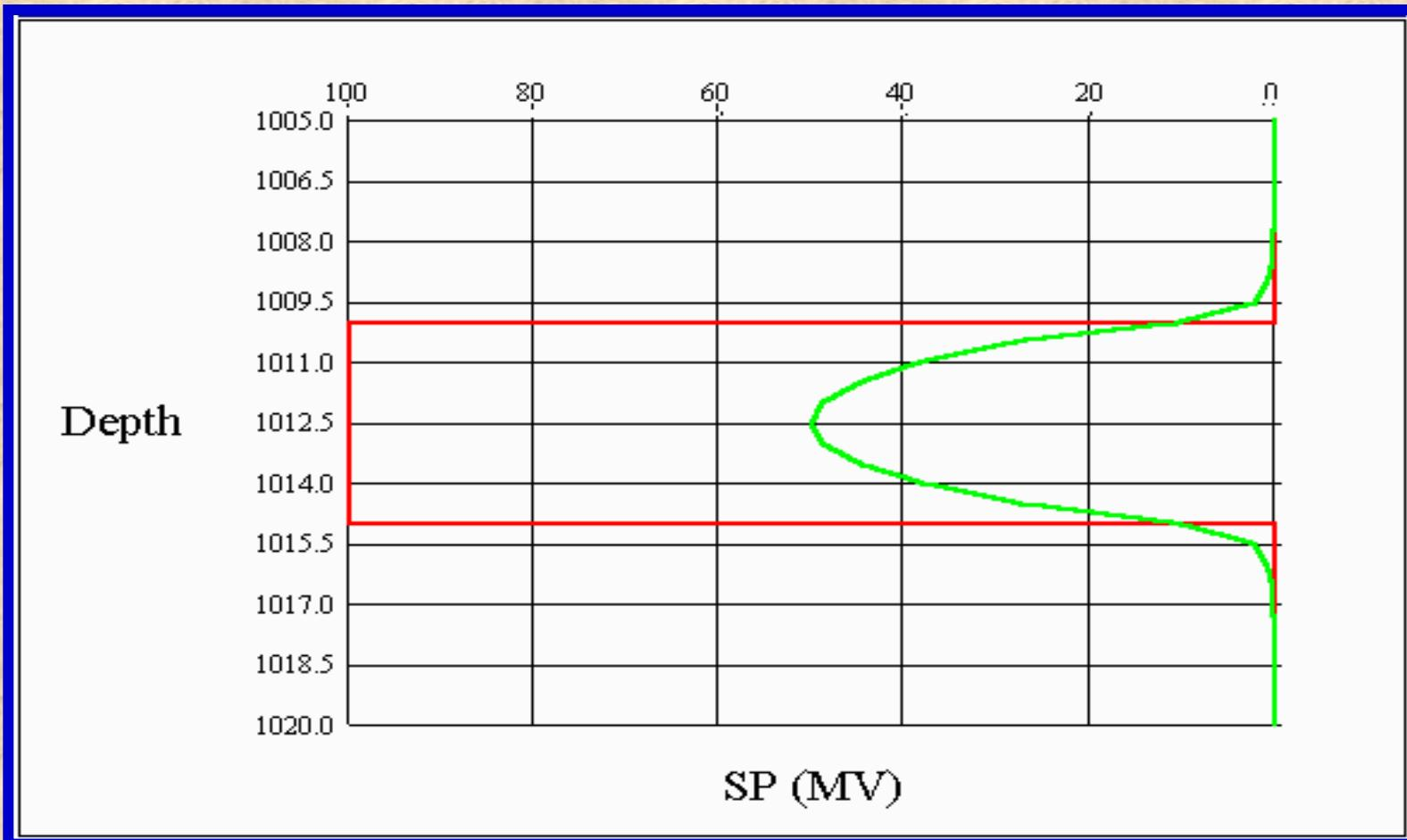
5 foot thick, 50 ohm-meter resistive bed
