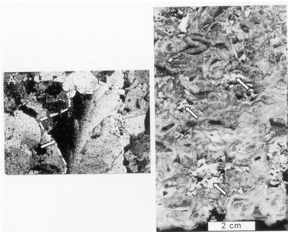
**Figure 14. Mesogenetic porosity. A - Thin-section photomicrograph of curved saddle dolomite (with typical undulose extinction) filling a pore. B - Core slab showing coarse crystalline saddle dolomite that has been partially dissolved to exhume (vuggy) porosity**
