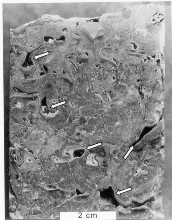
**Figure 4. Core slab with secondary vugs (arrows) resulting from the partial dissolution of earlier dolomite cement (white).**
