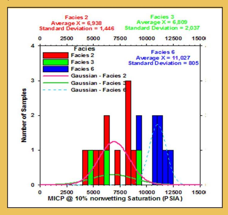
The distribution of measured capillary pressure values in the data set fits within the distribution of critical seal pressures (10% non-wetting phase saturation) from samples in other deepwater wells, analyzed to date.
