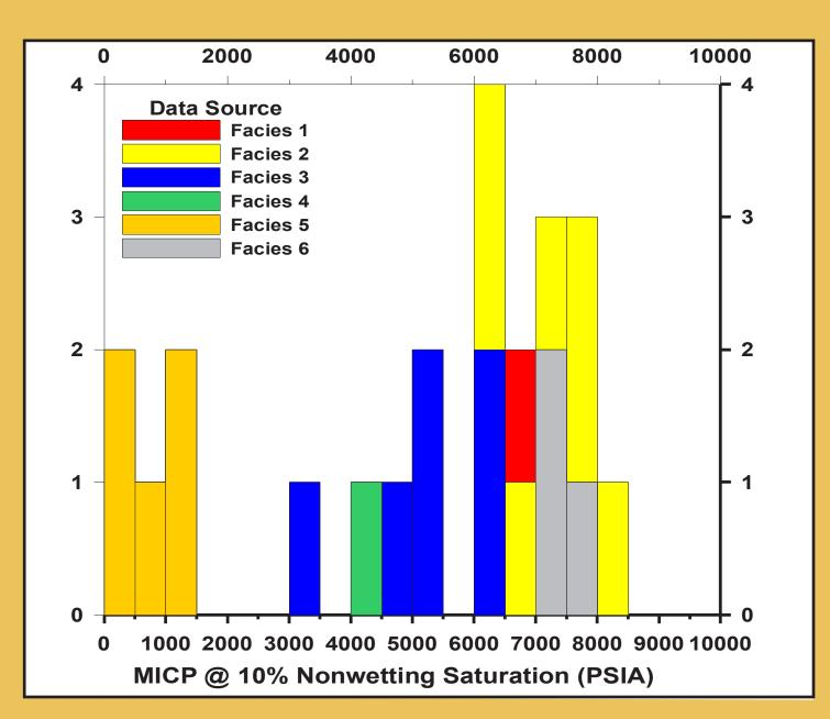
Shale types 1, 2, and 6 exhibit excellent top (membrane) seal potential. Silt-rich shales (types 3, 4 and 5) have considerably lower critical seal pressures.
