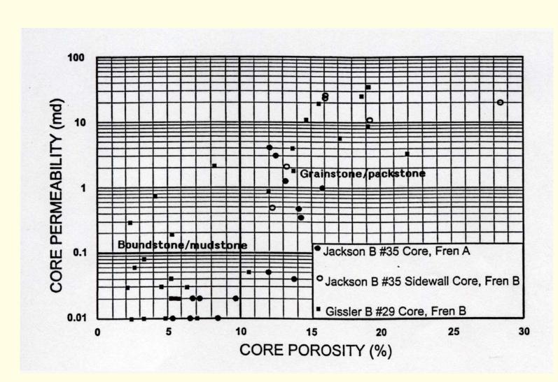
Plot of porosity vs. permeability for dolomite core plugs and sidewall cores from Jackson B #35 and Gissler B #29 wells. Only samples with permeability equal or greater than 0.01 md are included. Due to low permeability, "pay" porosity threshold is approximately 10%.
