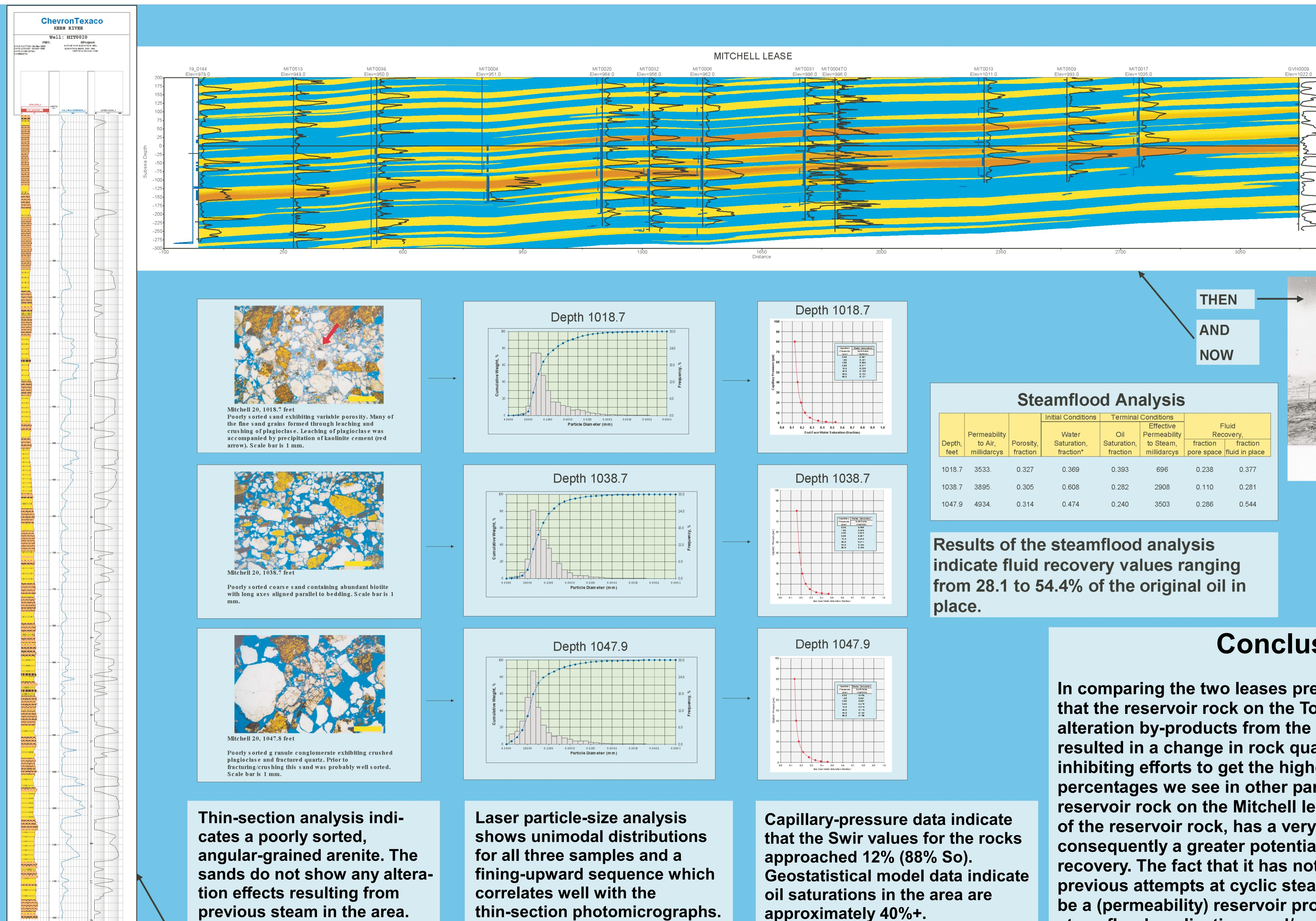
This log is showing, from left to right, the lithology (sandstone and siltstone), a resistivity curve, and a heat-corrected permeability curve based on the conductivity measurement. Thanks to Paul Harness, Formation Evaluation Specialist
