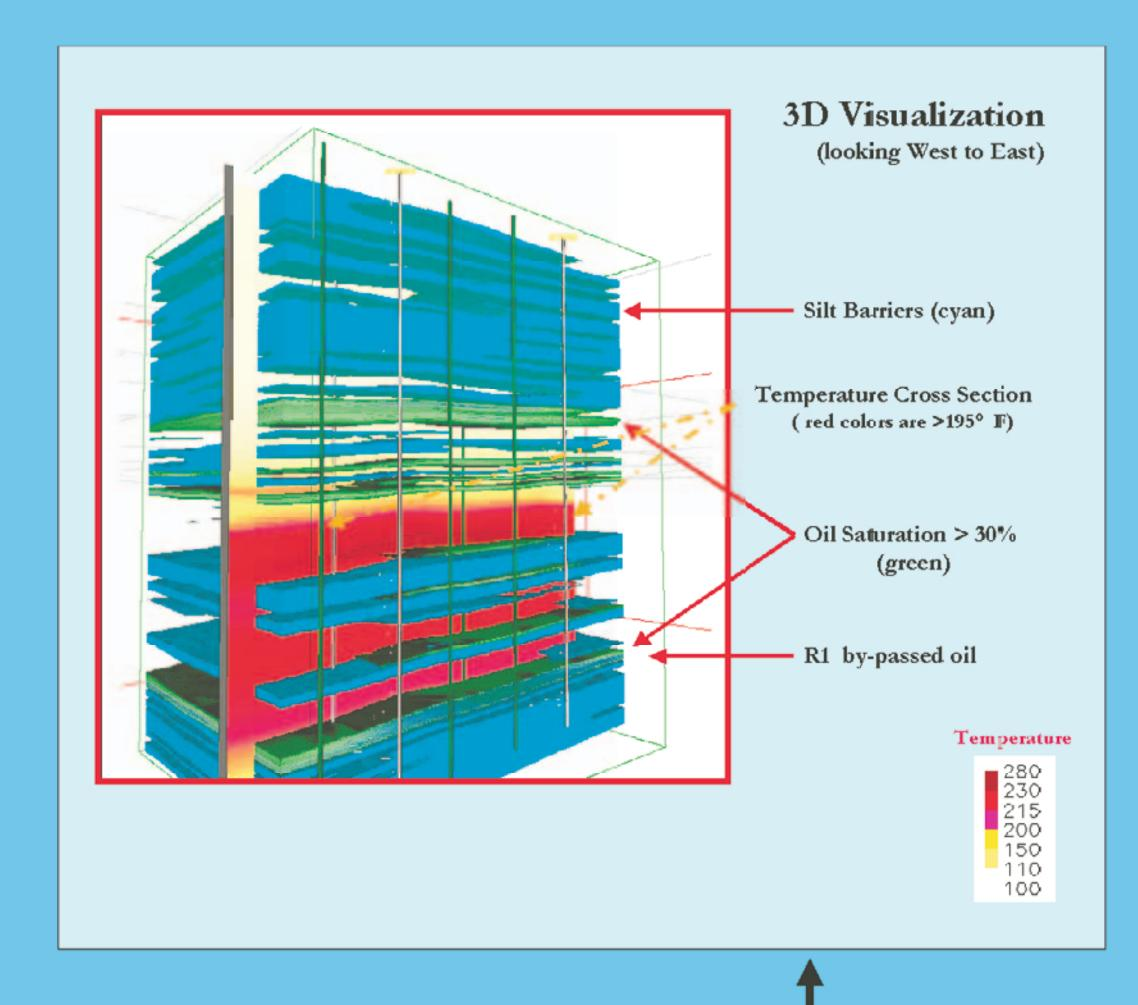
3D model of the KRF showing lithology, oil saturation, and reservoir temperature. This type of modeling is done routinely on a field-wide level down to the individual well level.
