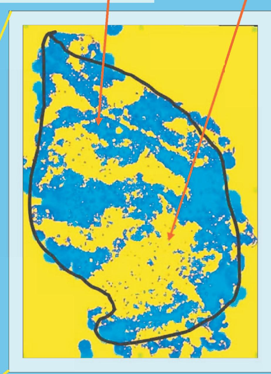
A horizontal slice through a 3D cube of resistivity data consisting of 9000+ log traces. Slicing down through these data reveals the channels, braided stream beds, and overbank deposits that make up the Kern River Formation (KRF).
