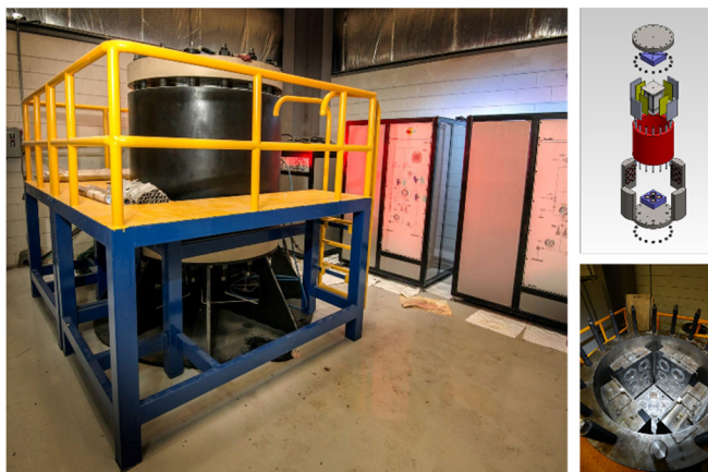
Fig. 3. True triaxial stress frame used to perform hydraulic fracturing block tests.
