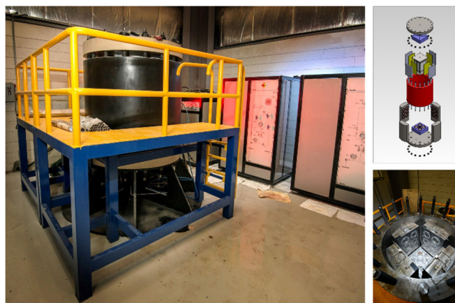
Fig. 4. True triaxial stress frame used to perform hydraulic fracturing block tests.
